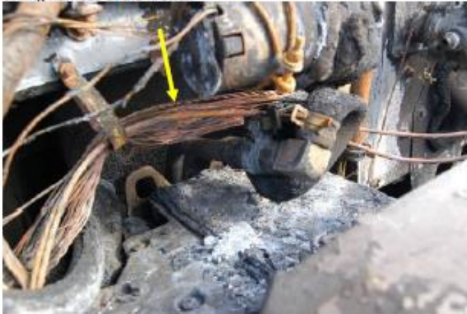
Photograph 4 Wiring harness at the firewall
