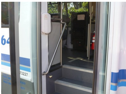
Front RFID antenna in paratransit bus
