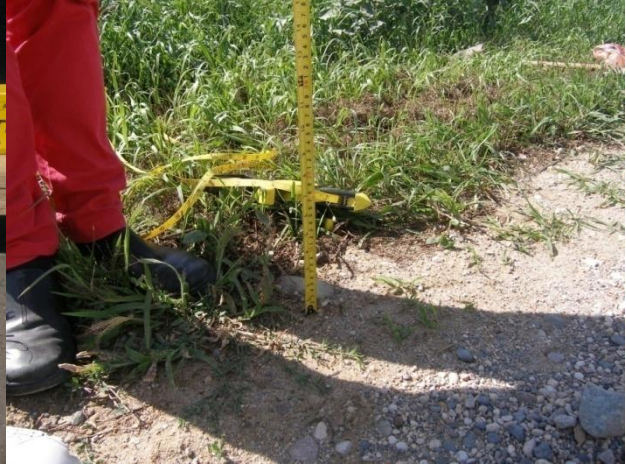
Measurement of cross section slope
