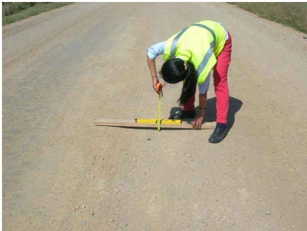
Measurement of pothole depth
