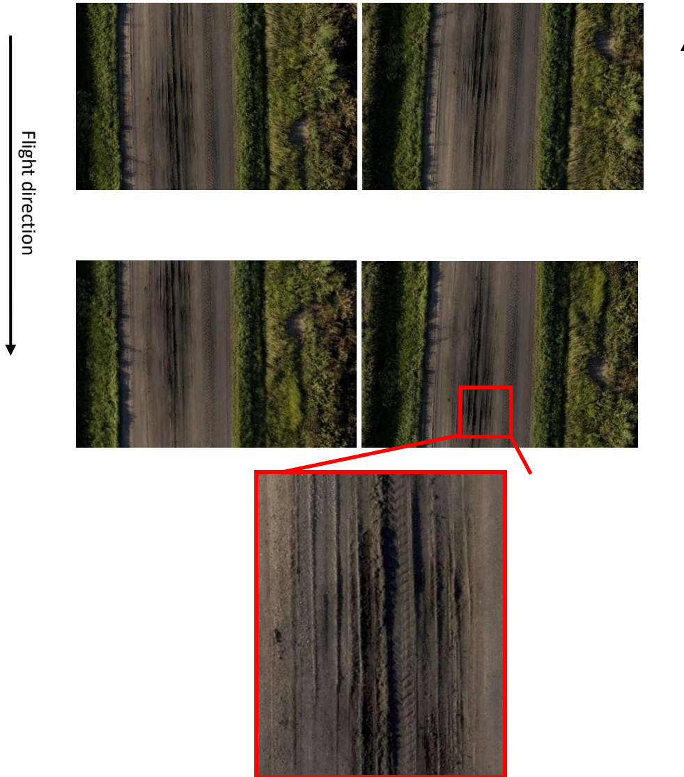
Figure 17. Example of road images acquired by UAV over a road segment. The segment was captured 4 times in a single mission. The flight directions are indicated by arrow lines. The bottom image shows the fine details of road feature (ruts) in original resolution.
