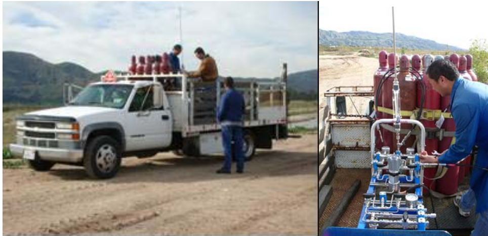
Figure 4 (left) shows the methane tanks used for the gas leak demonstration testing. Figure 5 (right) shows the methane release apparatus.
