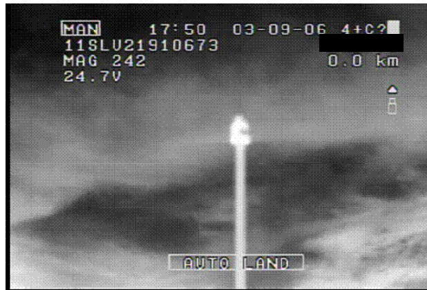
Figure 6: Infra-red image of methane release
