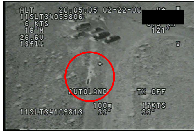
Figure 29: Infrared image of controlled heated inert liquid spill
