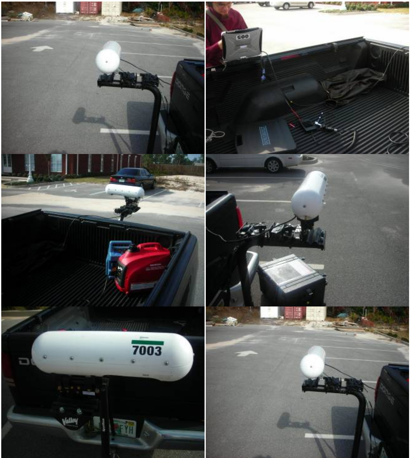
Figure 3.1-10. Ground-based testing of airborne sensor on truck mount.
