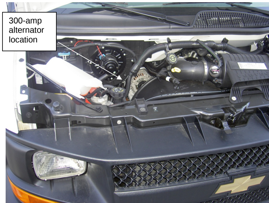
Figure 3.1-4. Integration of the 300-amp direct replacement alternator in ASAP van.
