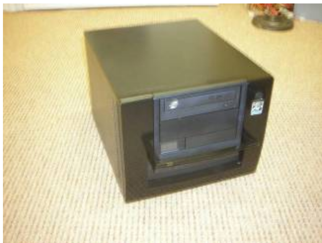
Figure 3.2-40. ASAP data control computer photograph (front panel shown).
