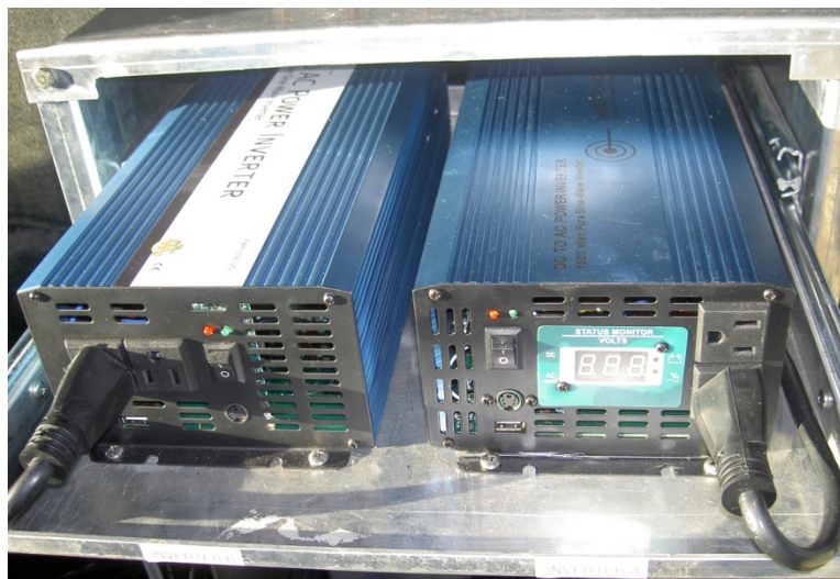
Figure 3.1-6. Photograph of two 1500 W, 115VAC, 60 Hz power inverters on equipment slide tray – slide out for access.
