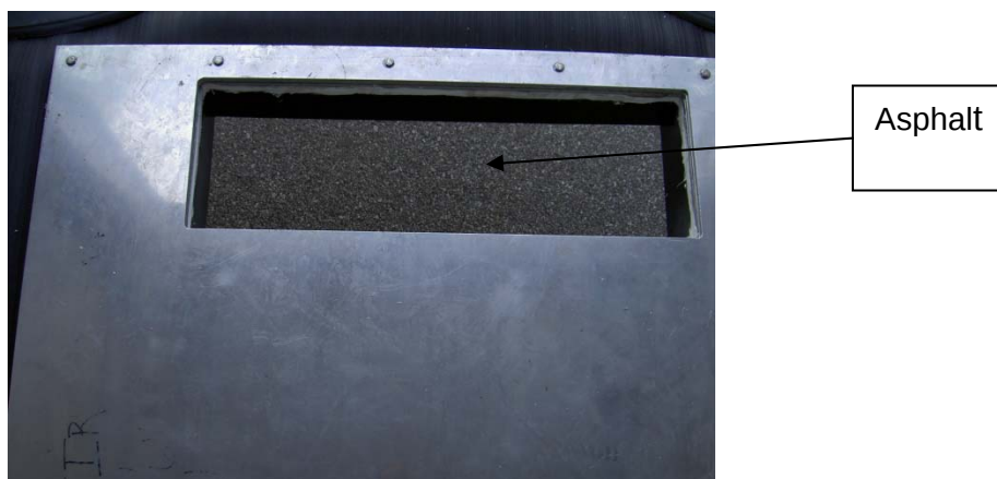
Figure 3.1-2c. Top down view of FTIR mount plates with door open.
