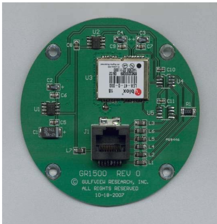
Figure 3.1-16. Integrated GPS/antenna board to support navigation of van for field testing.
