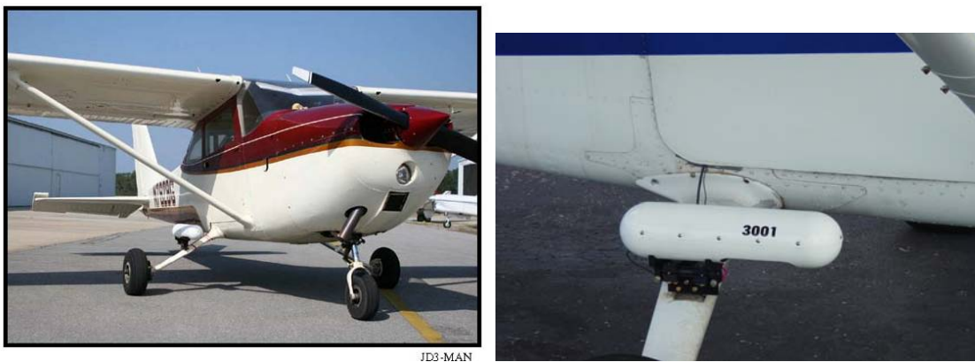
Figure 3.1-9. Airborne multispectral camera system mounted on Cessna.
