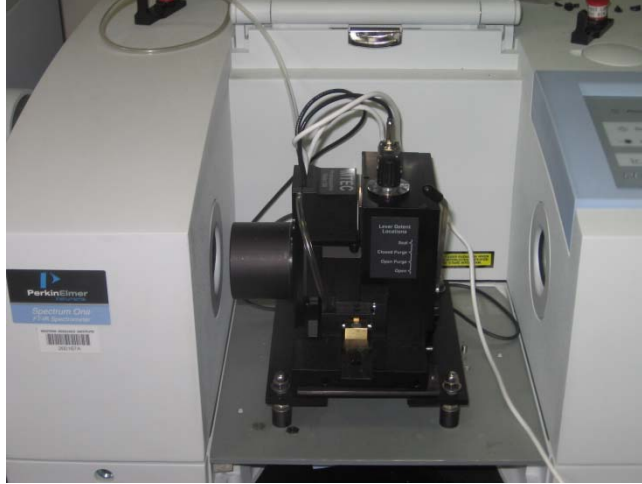
Figure 1.1-1. MTEC 300 Photoacoustic spectrometer coupled to a Perkin Elmer FTIR Spectrum One.
