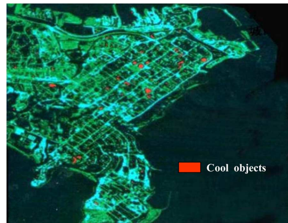
Fig. 19. Monitoring of cold energy leaks in Darwin, Australia using TIR wavelength bands data of MAIS sensor.
