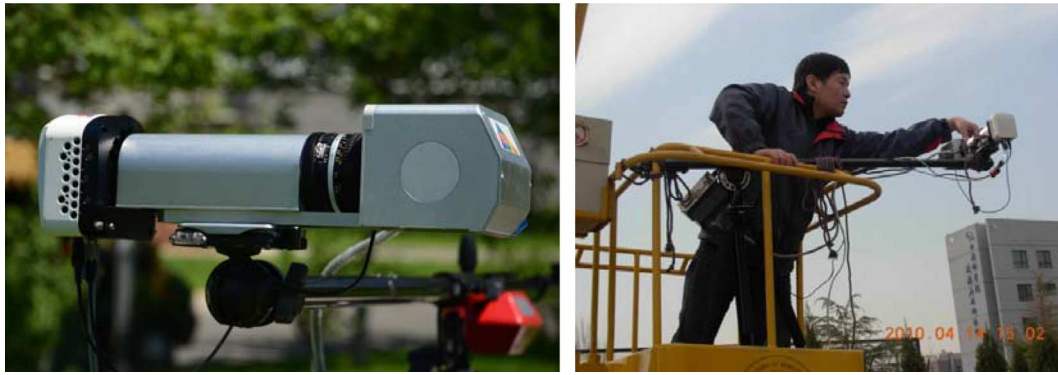
Fig. 4. The FISS at work: (left) situated on a ground-based multi-use platform and (right) mounted on an elevated car.
