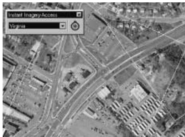
FIGURE 3 Northern Virginia's US-1 project plan with digital 1-ft resolution orthophoto and ArcView Fairfax County parcel information. The instant imagery access button is shown.
