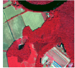
Portion of an AVIRIS scene with forest, bare and vegetated fields, and a river, shown with a color-infrared band combination (vegetation is red). Fraction images from linear unmixing are shown below.
