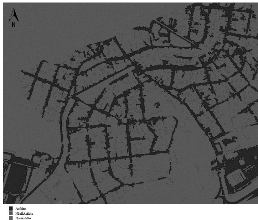
Figure 3 - Image with asphalt classifications resulting from the object-based classification algorithm (Asphalt=dark gray, Non-Asphalt=light gray and Asphalt Island=gray)
