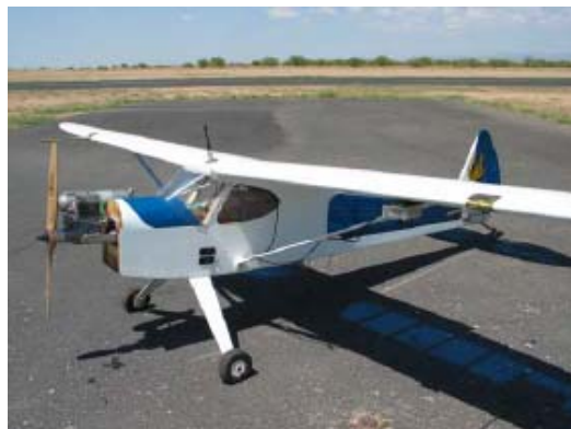
Figure 13: Experimental autonomous aircraft: Sig Rascal radio-controlled airplane
