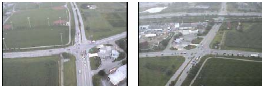
Figure 10: An example of circling a facility with the UAV, showing queue lengths and turning movements.
