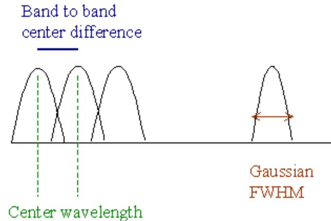
Spectral response modeled as a gaussian with a center wavelength and full width half max
