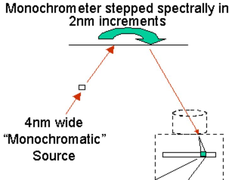
Monochromator profiles used to define center wavelength and bandwidth at discrete locations
