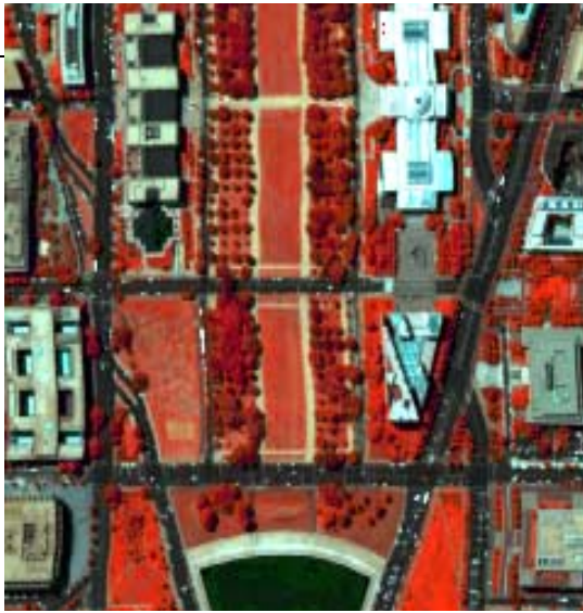
A simulated color IR image of an urban area, the Washington DC mall. This image is made using 3 bands of the 210 bands collected by the sensor system, one band from the visible green, one from the visible red, and one from the near infrared. Such displays are referred to as displays in image space .
