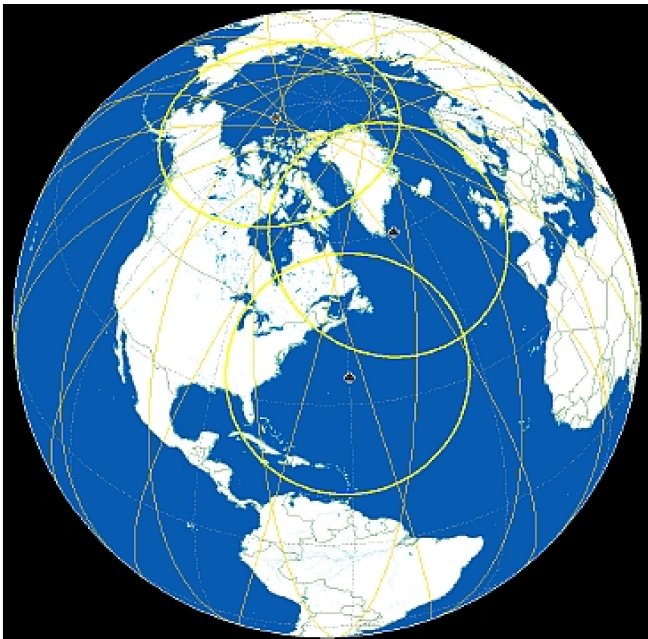
Figure 74: The circles show the typical IFOVs of a LEO satellite (image credit: COM DEV Ltd.)
