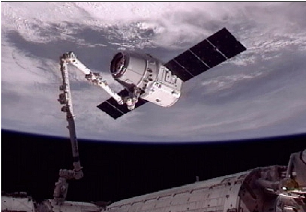
Figure 136: NASA TV snapshot of the Dragon capsule after it was captured by the robotic arm (image credit: NASA)
