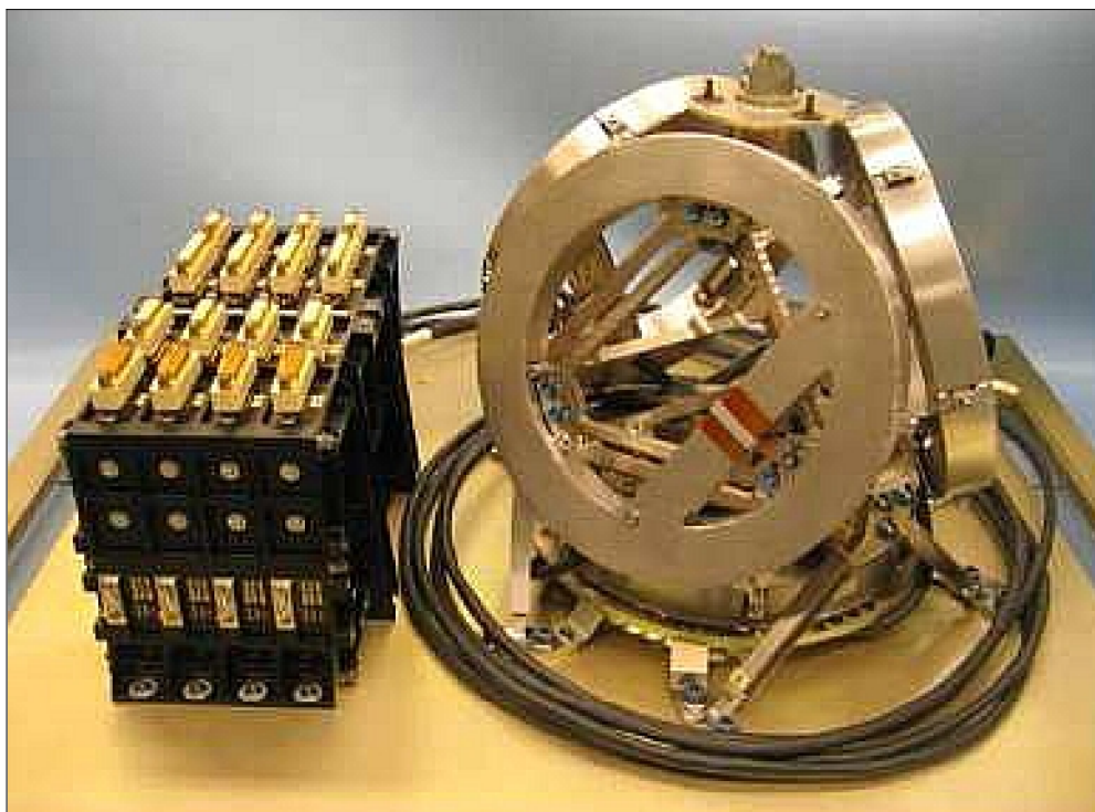
Figure 187: Astrix 200 FOG: coil size: 5 km, angular random walk: 0.0002^\circ/\text{hr} , scale factor stability: 30 ppm, 20 W, 7 kg, lifetime 5 years (image credit: ESA)
