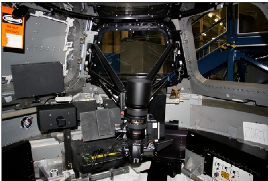
Figure 32: NightPOD installed on a mock–up of the European Cupola observatory during testing (image credit: ESA)
