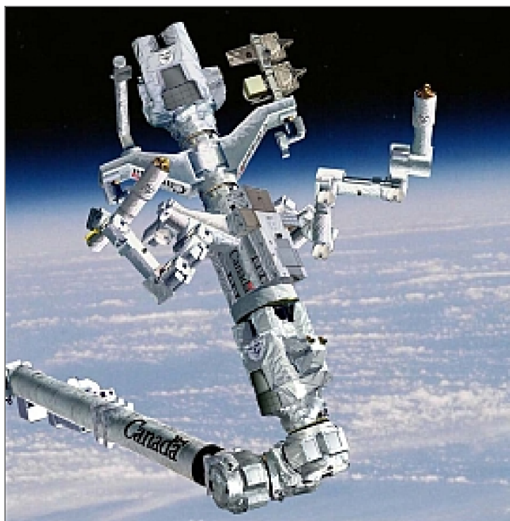
Figure 107: Artist's view of the Dextre manipulator arm in orbit (image credit: CSA, NASA)
