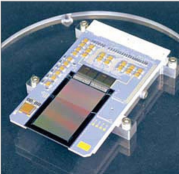
Figure 177: Prototype of the eROSITA pnCCD detector module with 2 cm x 2 cm large pnCCD (image credit: MPI–HLL)
