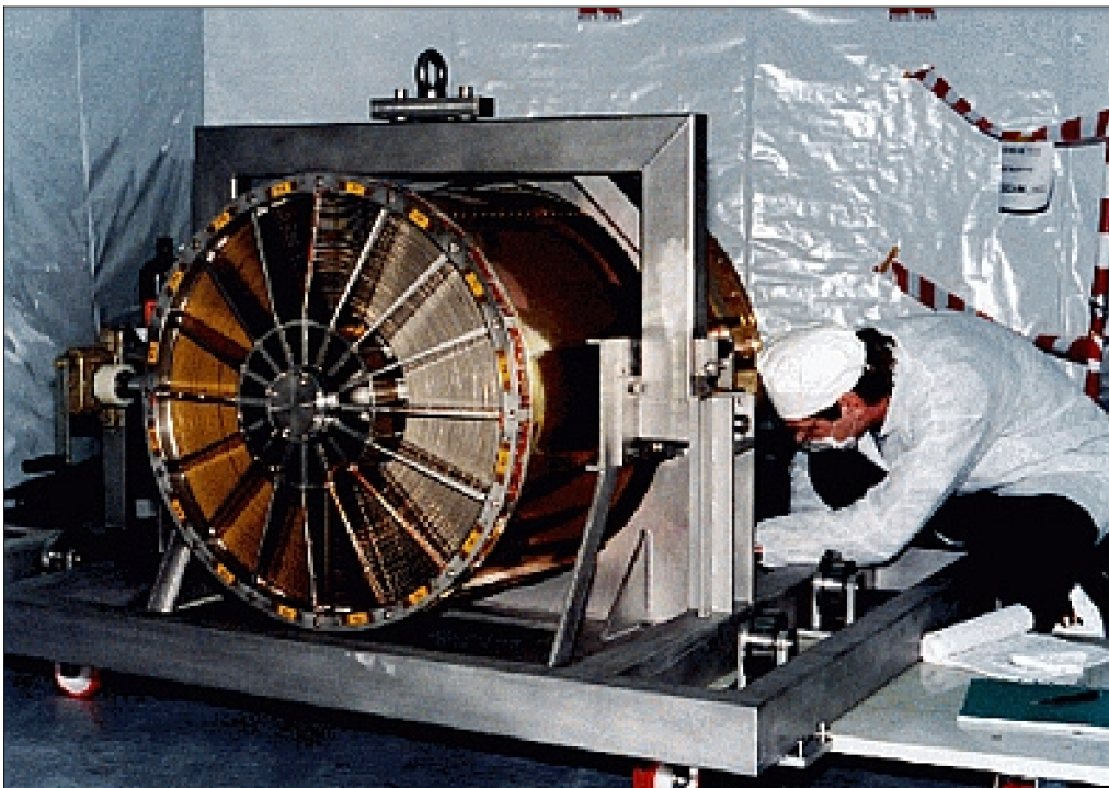
Figure 175: Curved mirrors stacked within one of three optical modules of the XMM–Newton telescope. Each one contains 58 mirrors with a total telescope optical surface of more than 120 \text{ m}^2 (image credit: ESA)
