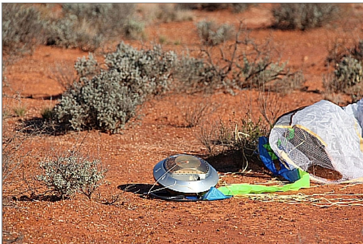
Figure 94: Photo of Hayabusa's sample return canister and parachute on the ground in the Australian outback (image credit: JAXA) 1634)
