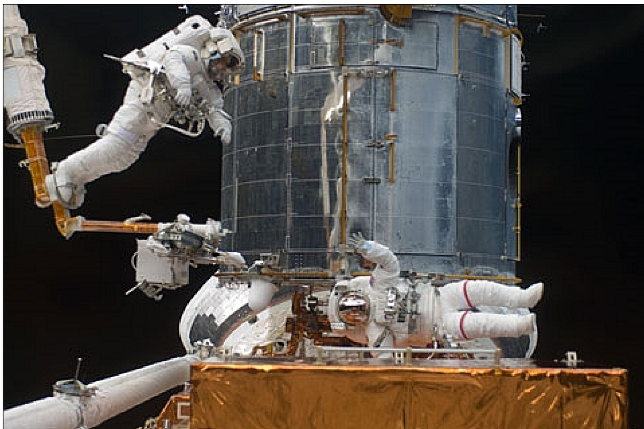
Figure 212: STS-125 astronauts navigate the exterior of the Hubble Space Telescope on the end of the remote manipulator system arm, controlled from inside Atlantis' crew cabin (image credit: NASA)
