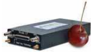
Fig. 4. PICCOLO LT Autopilot (CloudCap Inc., Accessed 2008).
