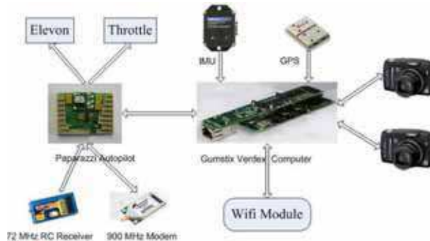
Fig. 8. AggieAir Airborne System Structure.
