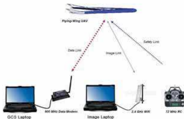
Fig. 6. AggieAir UAS Physical Structure.
