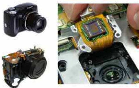
Fig. 9. Camera Body (left) and its CCD Sensor (right).
