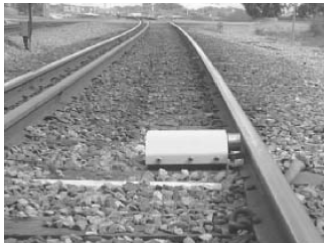
Figure 7-4: A mechanical sliding wheel detector
