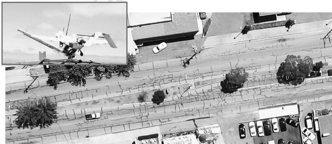
Fig. 8. UAV-based observation taken from a sensor platform shown in the upper left corner, for interpretations of road distresses over Gilroy, California (©MLB Company, http://www.spyplanes.com/ ).
