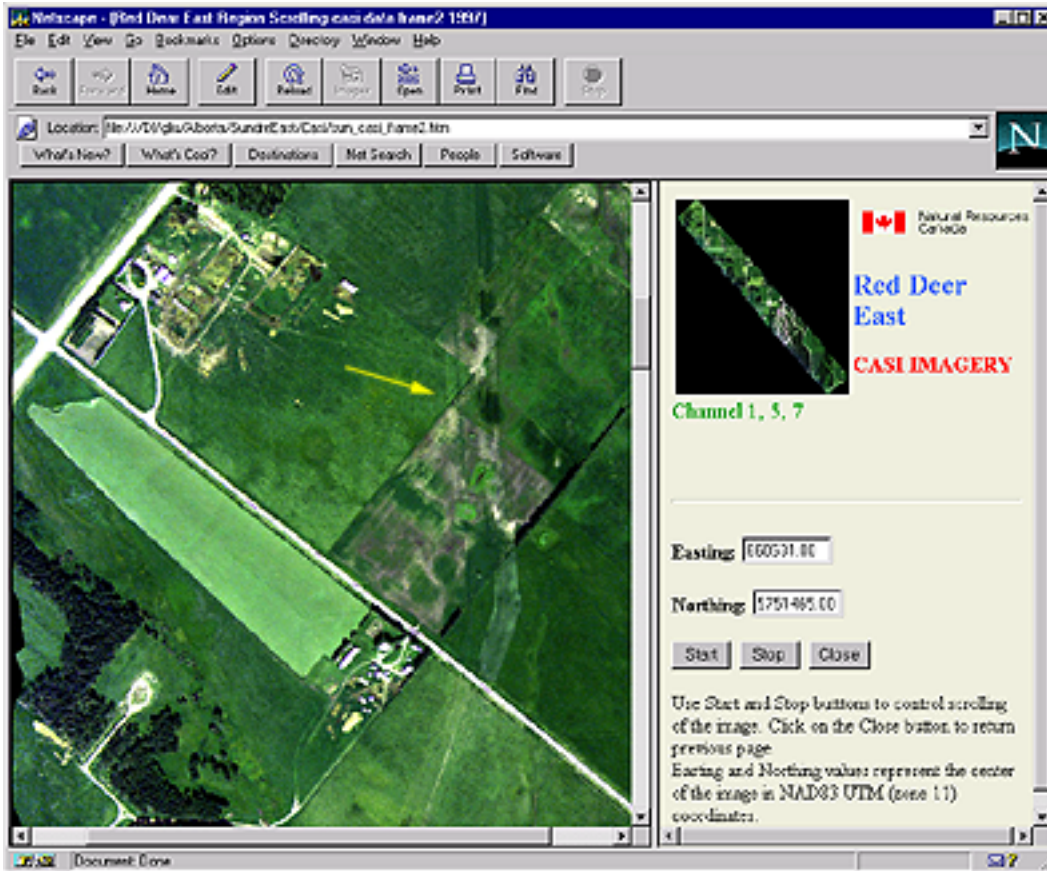
Figure 3. A screen capture of one of the web pages displaying a portion of the flight line in a scrolling window. The image was acquired using the casi instrument by ITRES in July 1997. Pointing by the yellow arrow is the Right-of-Way corridor.
