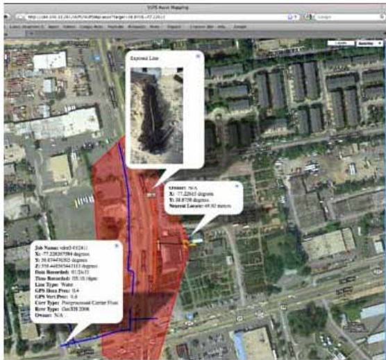
The One Call Ticket's proposed dig site area is plotted in the red polygon area. Current asset location data, equipment position as well as photo tags of the asset are readily accessible and readily viewed if they are available. The Google Satellite imagery feature has been selected.
