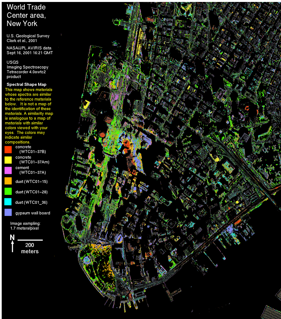
Figure 35. Analysis of Materials from Destruction of the World Trade Center in New York
