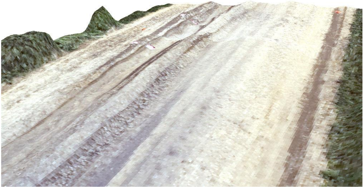
Figure 25. Reproduce of 3D image of road with severe distress from UAV-acquired imagery.
