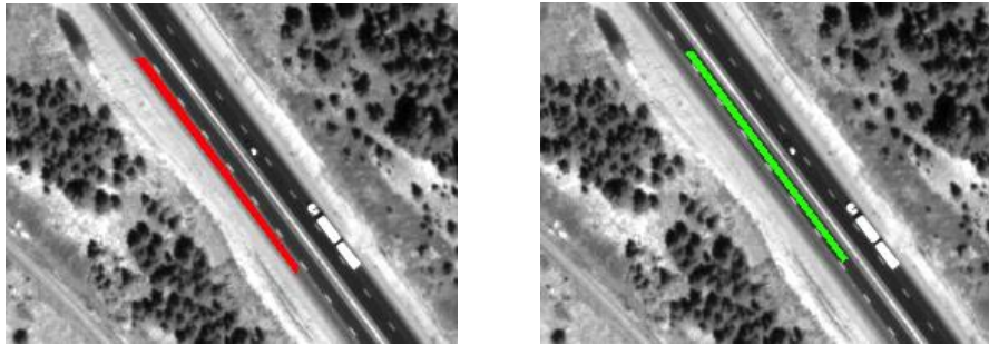
Fig. 16: Regions of interest for statistical computations of the poor road surface (red) on the left and the good road surface (green) on the right.
