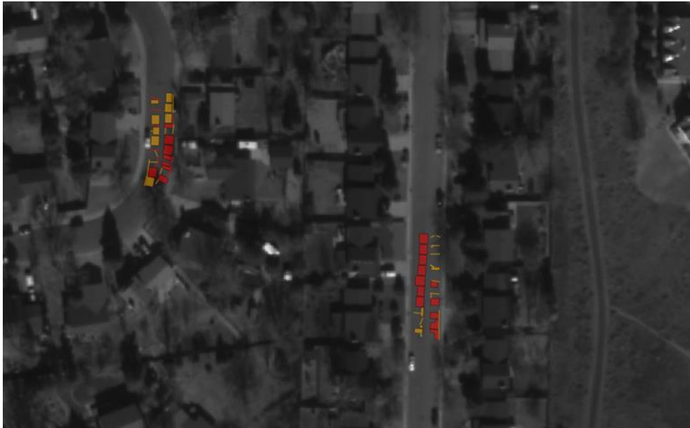
Figure 12: WorldView-2 Panchromatic Image with Road Damage Information
