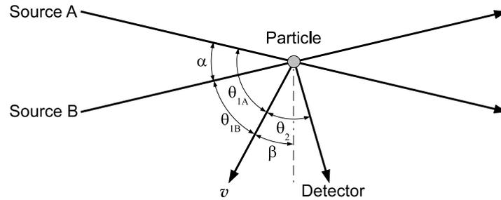
**Fig. 10.9** Geometry of the heterodyne detection method for laser Doppler velocimetry. Two laser beams, denoted sources A and B, cross at their focal points with angle  $\alpha$ . A particle passing through the beam-crossing region with velocity vector  $\mathbf{v}$  scatters light from both beams to the detector. Other angles are defined in the text.
