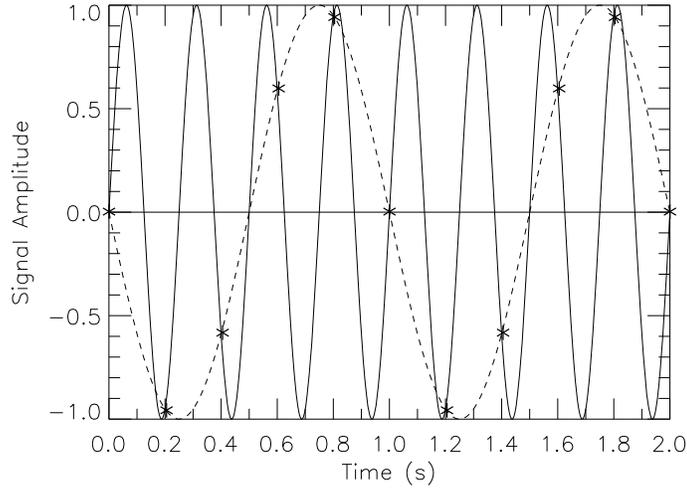
**Fig. 10.7** The aliasing effect: A sinusoidal signal with a frequency  $f = 4$  Hz is sampled with a frequency of  $f_s = 5$  Hz which violates the Nyquist theorem. The sampled points are represented as black stars and fit with a phase shifted signal with  $f = 1$  Hz.
