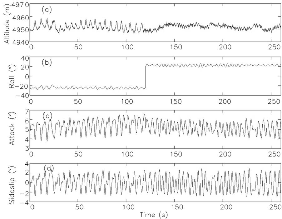
**Fig. 10.5** Time series of 10-Hz data from University of Wyoming King Air flight on 19 March 2009. Shown are section from left turn concatenated with section from right turn. Period of induced sideslip oscillations is 10 seconds.
