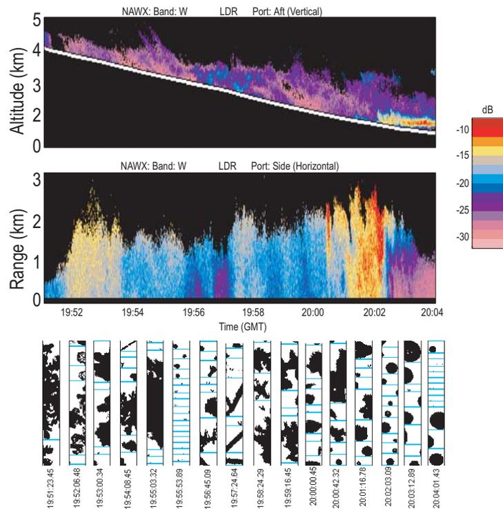
**Fig. 10.20** LDR measured by NAWX on Mar 01, 2007 as the aircraft descended from an altitude of 4 km to 1.5 km. Top: Vertical cross-section from upward pointing RADAR beam. The white line shows the aircraft altitude. Middle: LDR from the side-looking dual-pol antenna. Bottom: Sample of PMS 2D-C images corresponding to the aircraft altitude.
