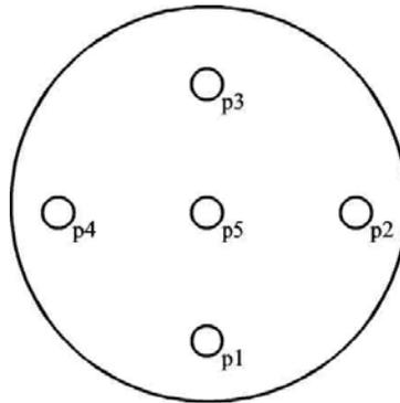
**Fig. 10.2** Schematic illustration of a FHP showing the pressure ports  $p_1$  to  $p_5$  (head-on perspective, i.e., starboard is on the left side from this point of view). In the text,  $p_0 = p_5$ .
