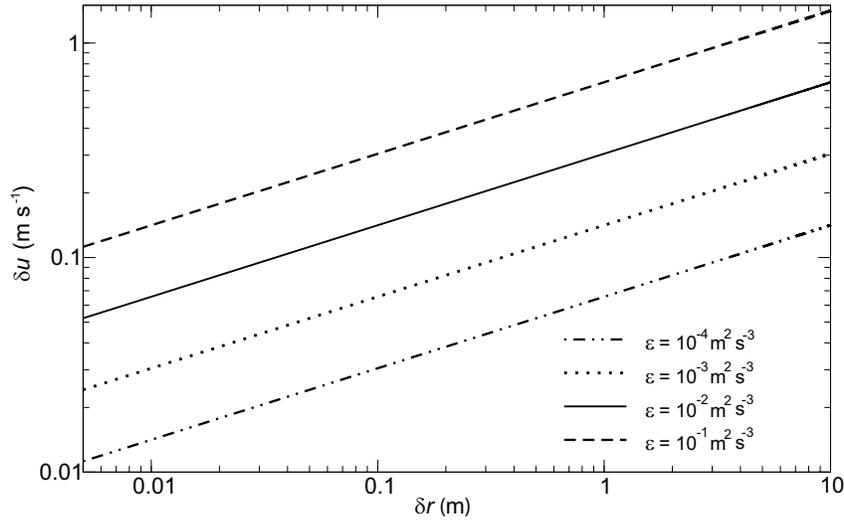
**Fig. 10.8** Required sensor resolution  $\delta u$  for velocity measurements as a function of spatial resolution  $\delta r = TAS/f_s$  and for different levels of turbulence described by the mean energy dissipation rate  $\epsilon$ .
