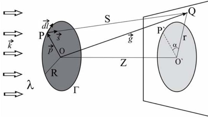
**Fig. 10.11** A schematic explaining calculation of diffraction by an opaque disc.
