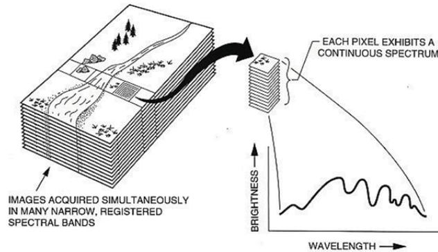
**Fig. 8.1** The concept of HRS/IS: Each pixel element has a continuous spectrum that is used to analyze the surface and atmosphere
