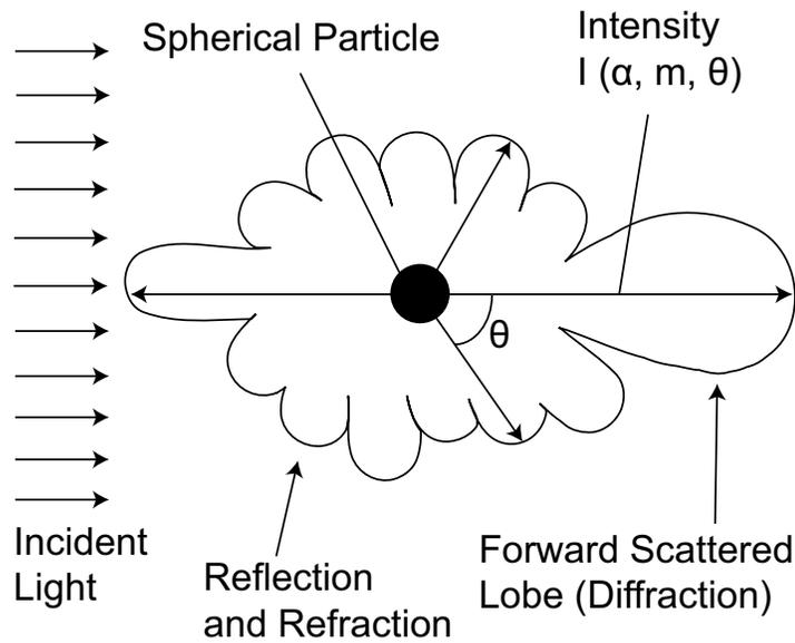
**Fig. 10.10** This diagram demonstrates the intensity of scattered light as a function of angle with respect to the incident ray for a typical spherical particle.
