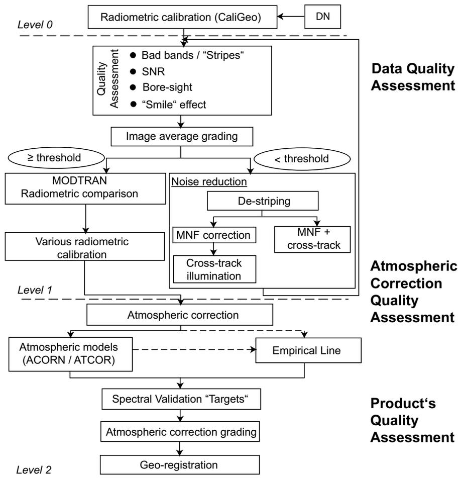
**Fig. 8.3** A data processing chain, as used at RSL-TAU (Remote Sensing Laboratory at Tel Aviv University) with the AISA-Dual sensor. Note that at three stages, quality assurance is crucial: the raw data (including radiance), the atmospheric correction stage (reflectance and emittance) and the thematic mapping stage.
