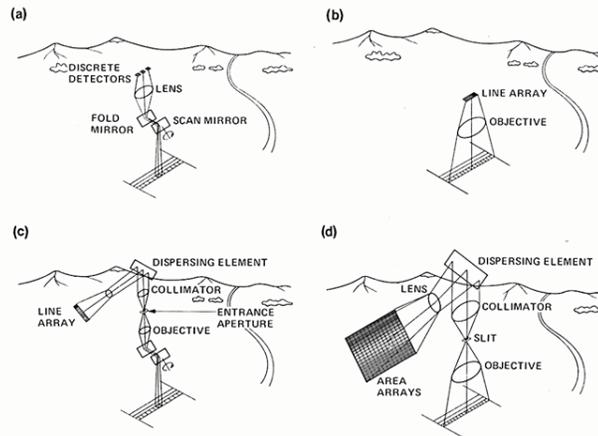
**Fig. 8.2** Four approaches to sensors for multispectral imaging: (a) multispectral imaging with discrete detectors (LANDSAT type); (b) multispectral imaging with line arrays (SPOT type); (c) imaging spectroscopy with line arrays (AVIRIS type, whiskbroom); (d) imaging spectroscopy with area array (AISA type, pushbroom).
