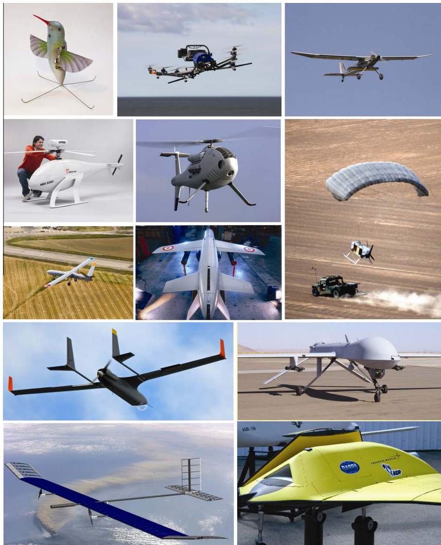
Fig. 1. From top to bottom, left to right, each picture illustrates a UAV of each category in van Blyenburgh (2013): AeroVironment, USA—Nano-Hummingbird; Ascending Technologies GmbH, Germany—Falcon 8; CATUAV, Spain—Argos; Swiss UAV, Switzerland—Neo s300; Schiebel, Austria—Camcopter S100; MMIST, Canada—Snowgoose; Thales, UK—Watchkeeper; Selex ES, Italy—Nibbio; Insitu Inc., USA—Integrator; General Atomics Aeronautical Systems, USA—Predator A; QinetiQ, UK—Zephyr; Lockheed Martin, USA—Morphing UAS.
