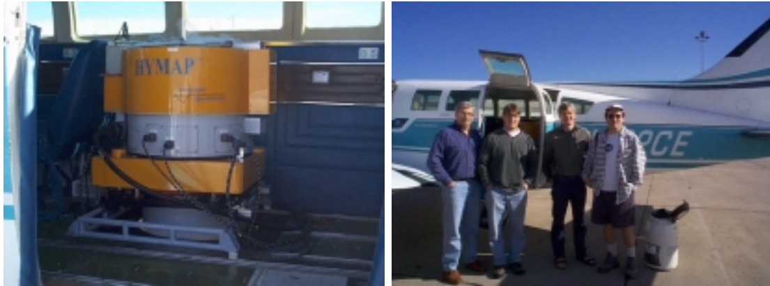
Figure 1. The HyMap sensor (left) and aircraft used for the USA acquisitions (a Cessna 402) and part of the HyVista/AIG team (right).
