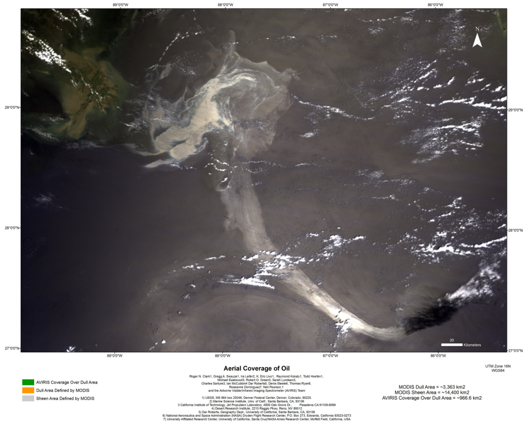
Figure 16a. Image of the spectral response from the oil spill area on May 17, 2010, from MODIS on the Terra Satellite. Lighter gray areas are interpreted to be sun glint reflecting off of the oil spill. See separate high-resolution jpeg file.
