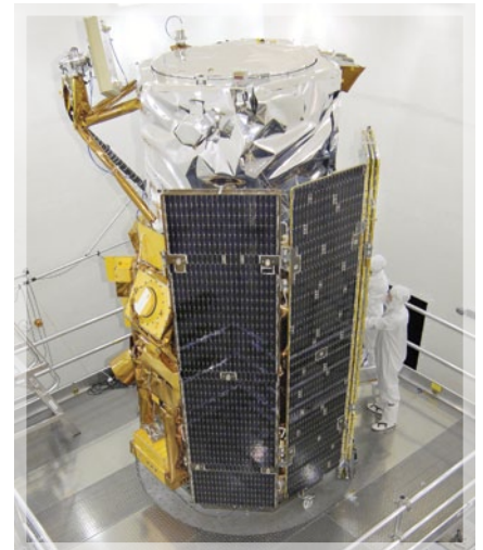
This photo of GeoEye-1 was taken from General Dynamic’s facility in Gilbert, AZ in May 2008. The photo shows test engineers in the clean room after successful completion of all environmental testing on GeoEye-1, which is an important step prior to being shipped to the launch pad.
