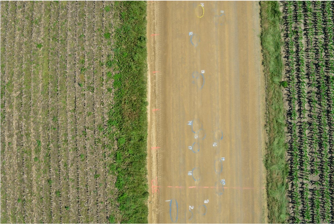
Figure 33: Part of Fleming Road segment 2 with marked, numbered distresses as captured by the MTRI hexacopter flying the Nikon D800 DSLR camera. Data were collected the day after the road was marked. Note the blue distress feature markings have been worn by passing traffic. Feature numbers were refreshed with white marking paint.
