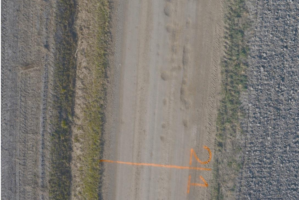
Figure 22: Aerial view of Piotter Hwy from the MTRI hexacopter flown at 25 meters altitude. Note the segment markings and clearly visible distresses (potholes) in the road surface. (DSC3227_gamma.jpg)
