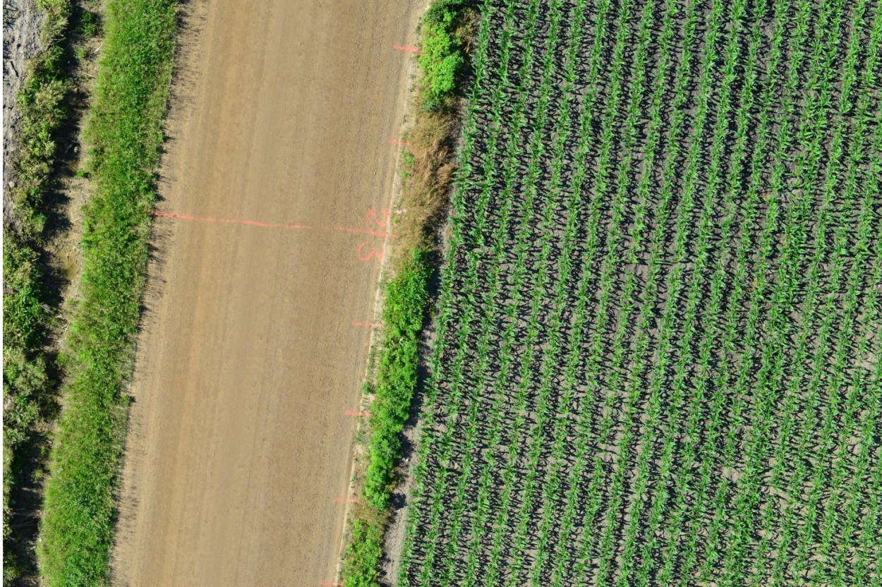
Figure 31: A segment of Marsh Road from the MTRI hexacopter. No significant distresses were present, however crown measurements were taken on Marsh Road for comparison to the results from image processing.
