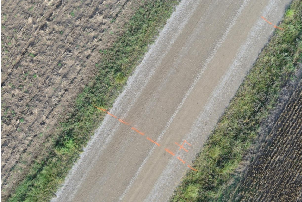
Figure 19: Aerial view of same segment of Mills-Macon Road as Figure 18 above, seen from the MTRI remote control helicopter flying at 25 meters above the ground. Note the road segmentation marks and slight windrowing of the loose aggregate on the road surface. (DSC3440)
