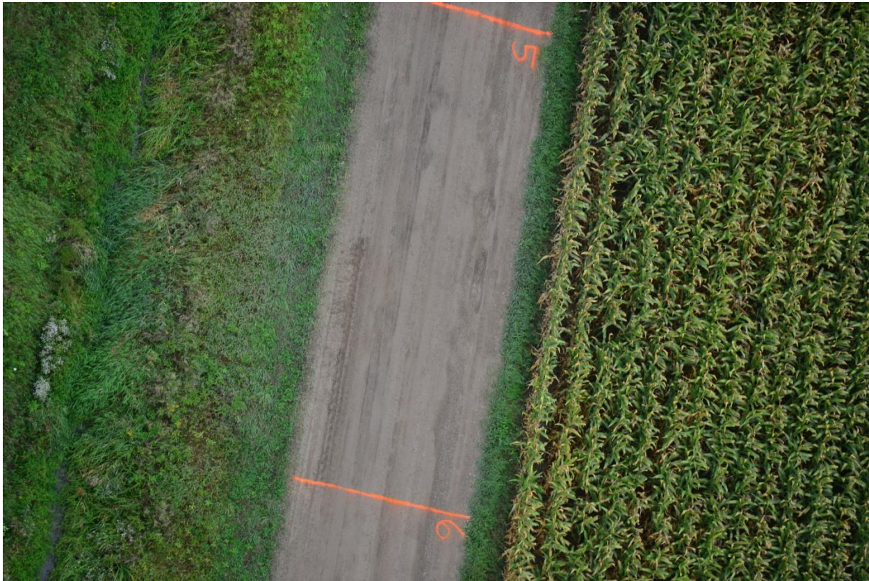
Figure 37: An image of an approximately 50 foot / 15 meter section of Palmer Hwy taken with the Nikon D800 camera with a 200mm lens from the manned Cessna 172 flight. Altitude and airspeed can make it difficult to capture usable overlapping aerial imagery from a manned fixed wing aircraft at a reasonable cost. (CJR_4426.jpg)
