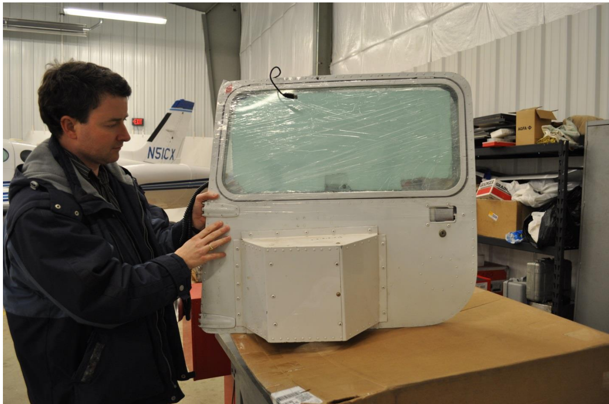
Figure 42: The door of a Cessna 152 with a fairing allowing the mounting of a camera pointed straight down (nadir).
