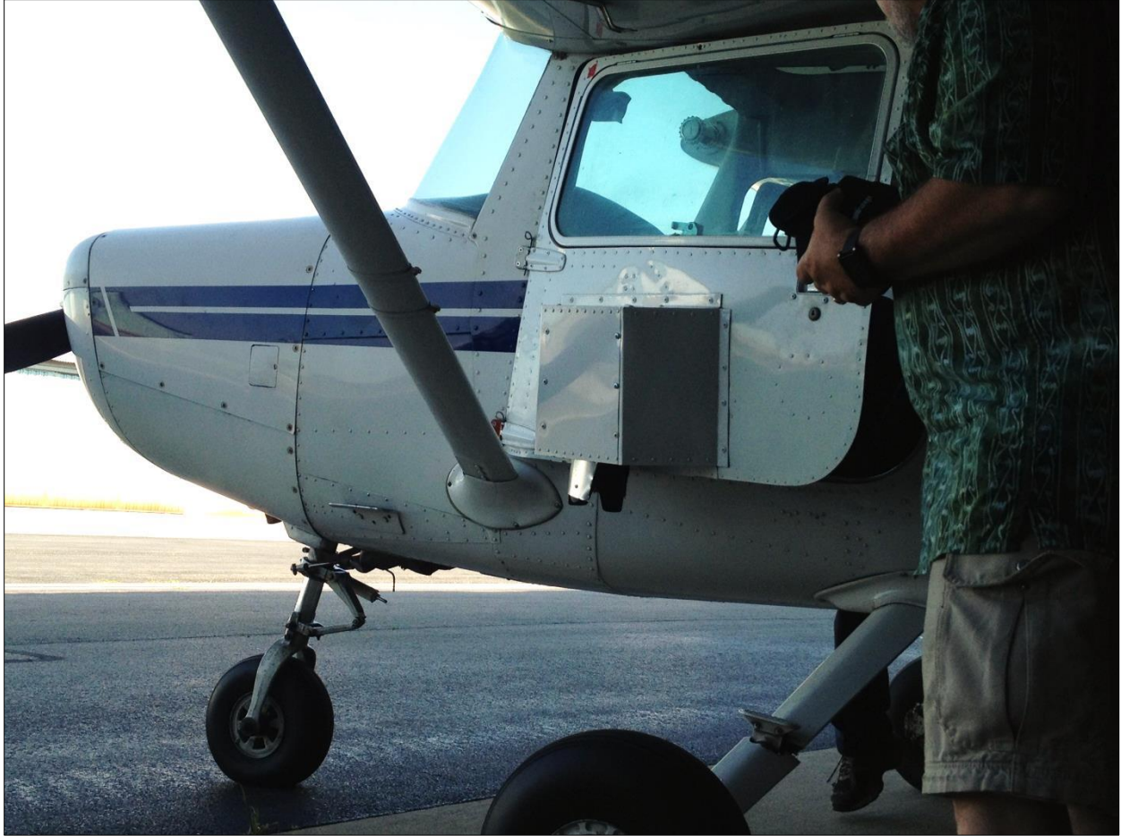
Figure 43: The Nikon D800 camera mounted on the door of a Cessna 152. The protective shade at the end of the camera lens can be seen at the bottom of the door.
