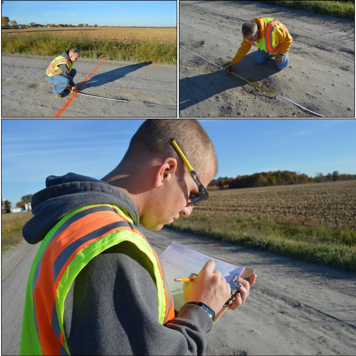
Figure 13: Location and attribute data about distresses found in each road segment were measured and recorded for comparison to image processing results. (three photos above): (DSC1285, DSC1295, DSC1297)
