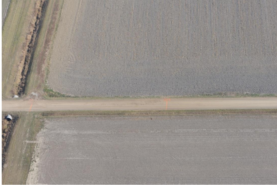
Figure 24: Low oblique aerial photograph of Piotter Hwy segment 2 from the Cessna 172. Markings are clearly visible but distresses while visible are too small to be characterized into classes based on size. (DSC5855)
