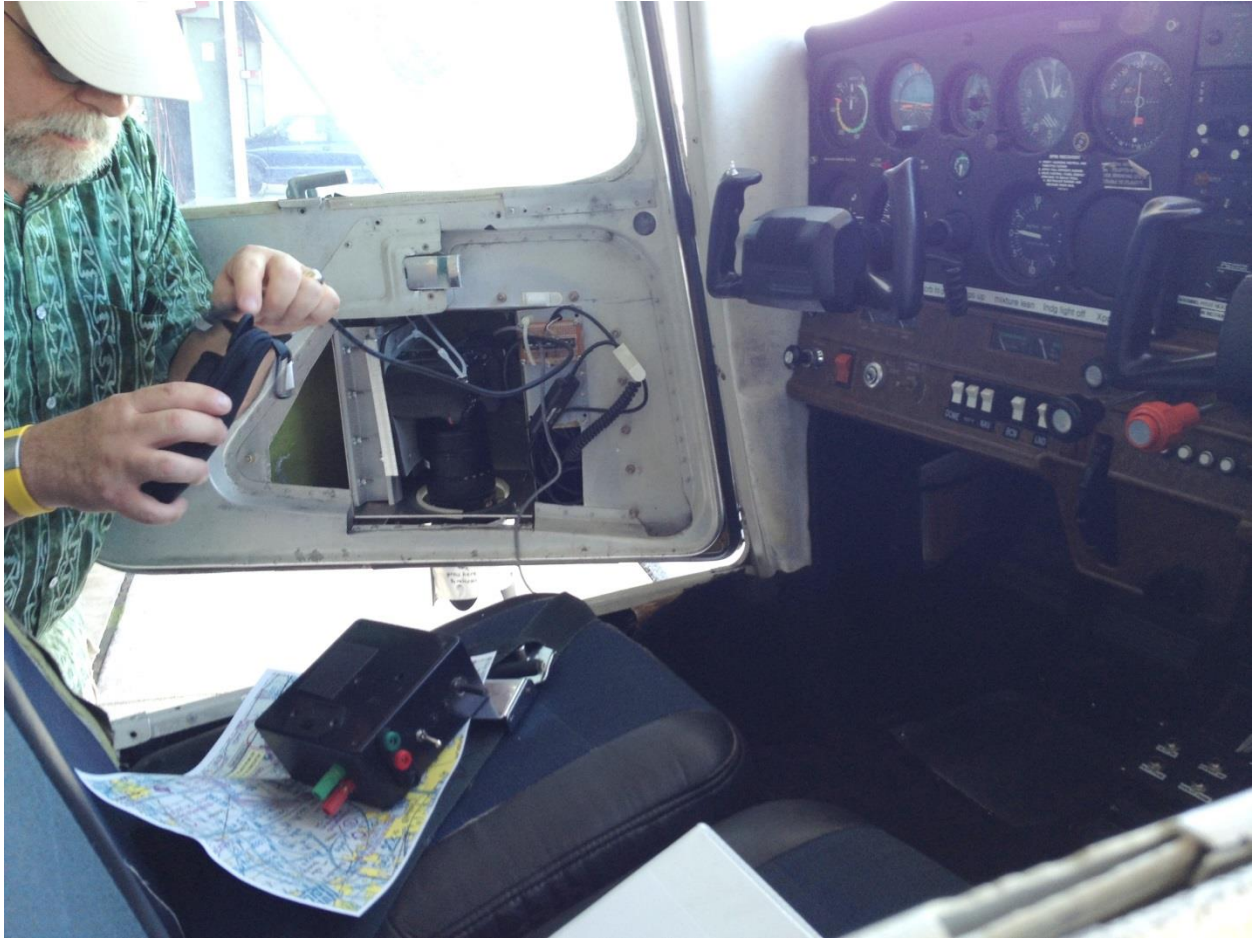
Figure 44: Preparing to fly the D800 in the door of the Cessna 152. The camera can be seen in the door, the camera trigger mechanism can be seen on the pilot seat.
