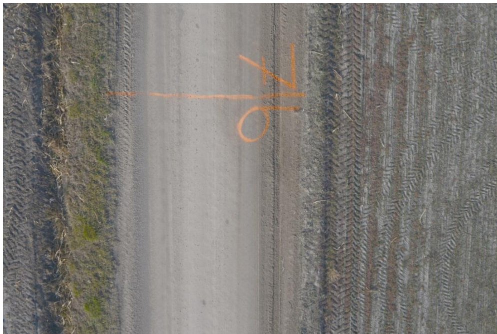
Figure 21: The same segment of Piotter Hwy seen in Figure 20 above from the MTRI remote control helicopter flown at 25 meters. Few potholes are visible in this image but a long rut on the right side of the road is visible in both this image and the ground view of the same area. (DSC3449_gamma.jpg)
