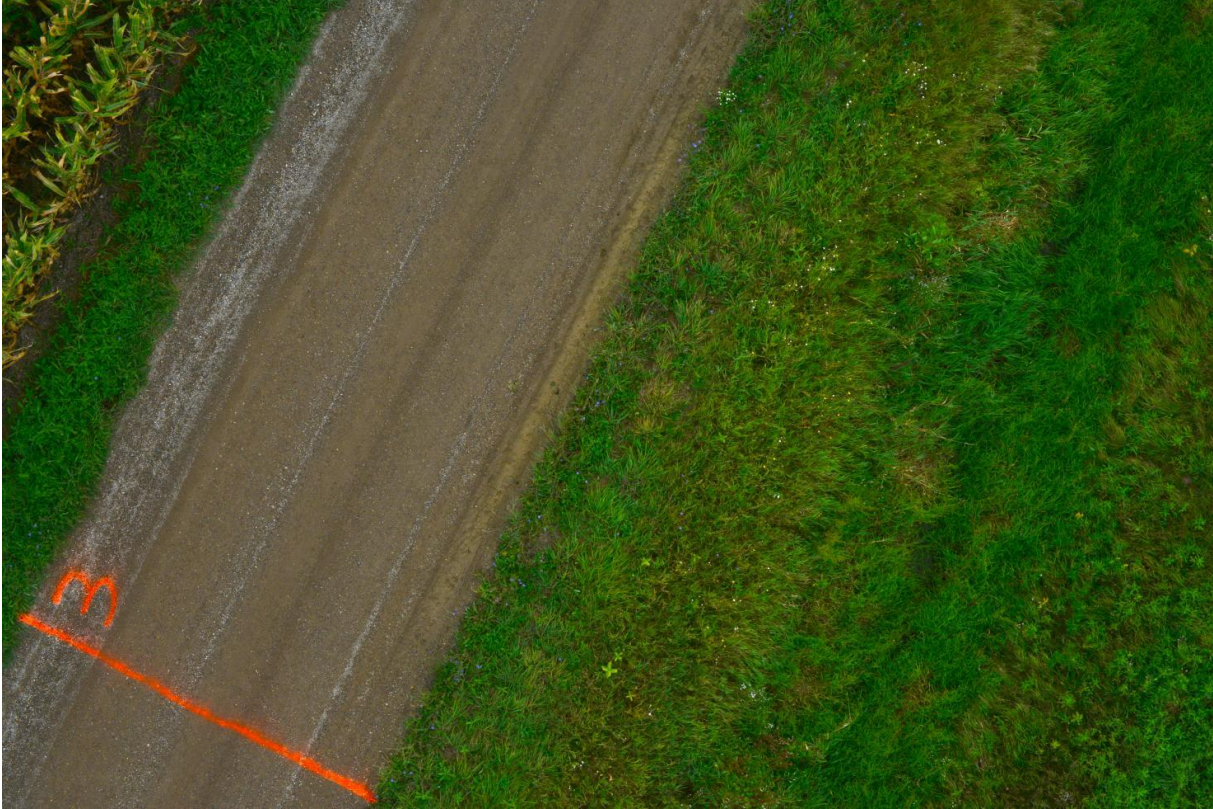
Figure 38: Segment 3 of Palmer Road from the MTRI hexacopter from approximately 25 meters altitude. A rut is visible on the right side of the road just above the segment line.
