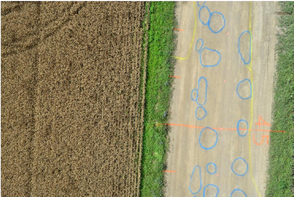
Figure 36: An image of Piotter Hwy from the hexacopter flight. This is approximately the same location as in the previous figure. Above, however the hexacopter flight was made before the distress features were numbered. (975-7916.jpg)
