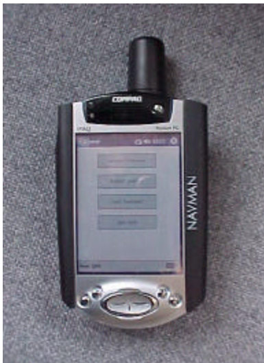
Figure 2.1 – The Compaq iPAQ™ 3538 equipped with a NavMan™ GPS 3000 receiver
