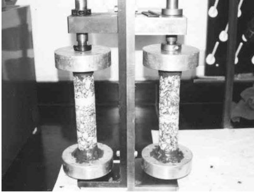
Figure 4.5 Mounting of TSRST Samples.
