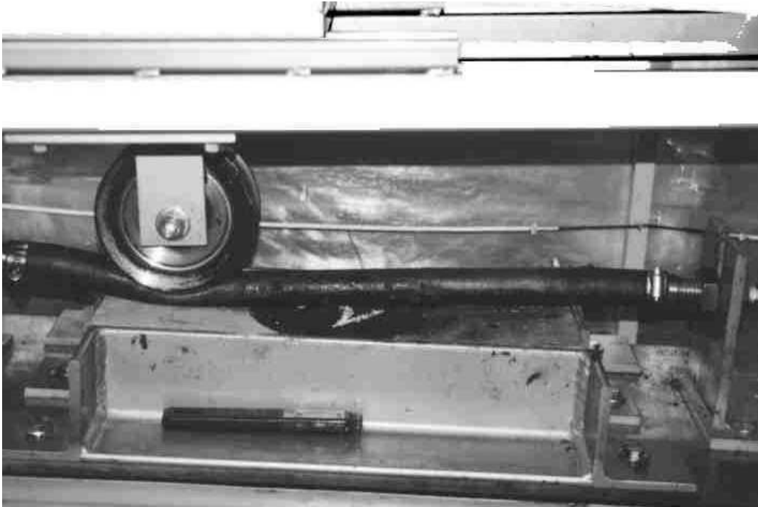
Figure 4.4 Sample Being Tested Using Georgia Loaded Wheel Tester.
