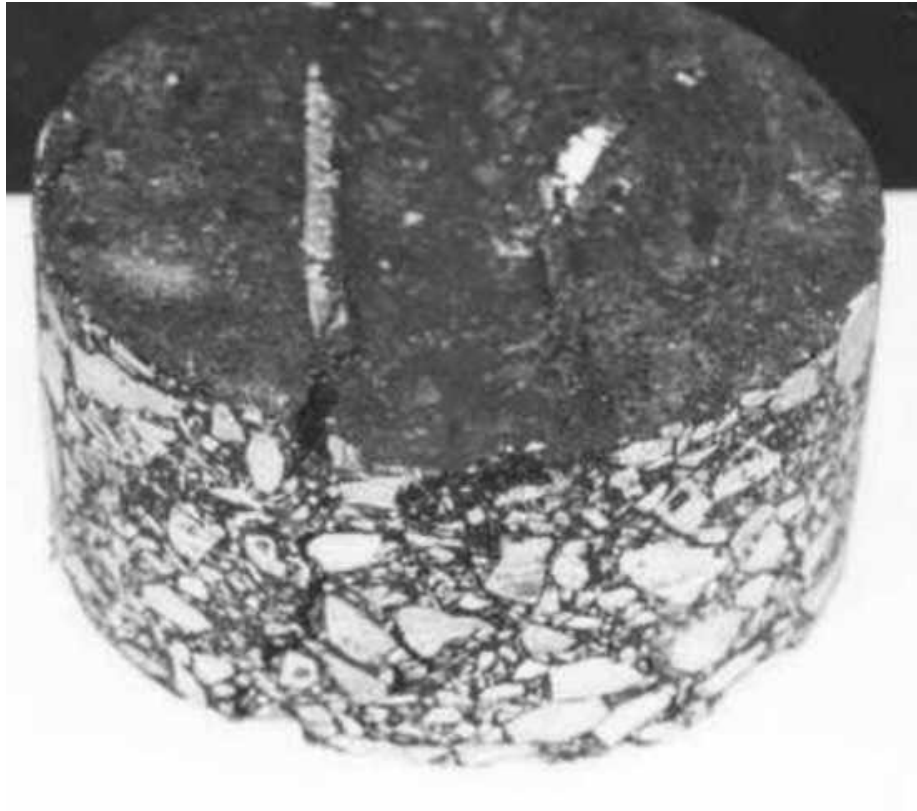
Figure 4.10 Failed GLWT Core Sample.
