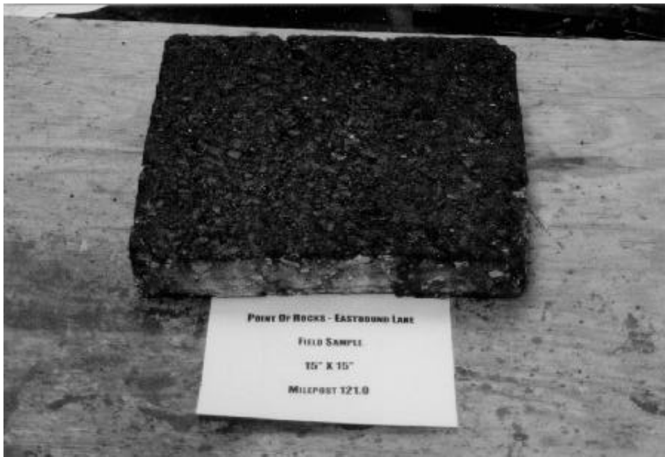
Figure 3.2 Pavement Slab Taken from Point of Rocks Project
