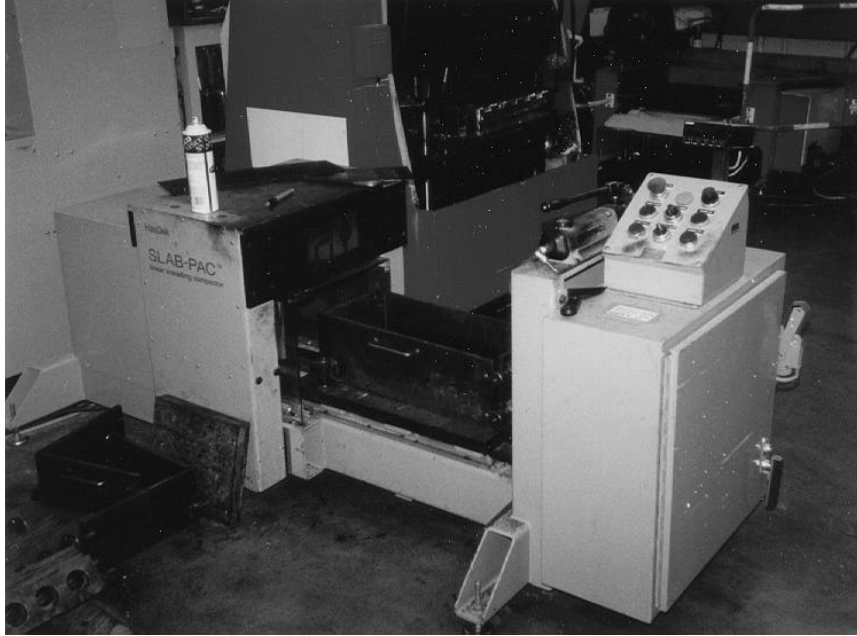
Figure 4.2 Linear Kneading Compactor located at CDOT
