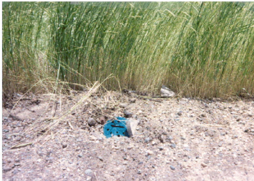
Figure 8. Runoff Sampling Container Installed at Shoulder of Road
