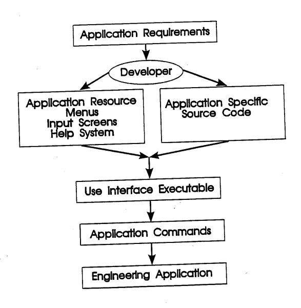
Figure 2. Architecture of User Interface
