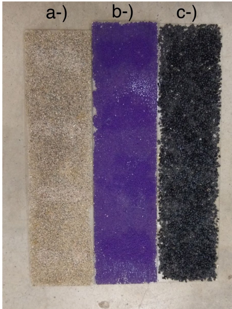
Figure 2.4 Various channel bed materials used: (a) sand, (b) glass beads, and (c) gravel
