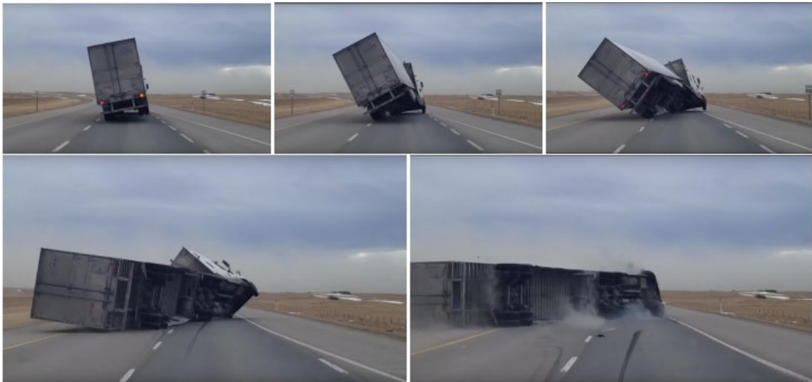
Figure 1.1 Sequence of a high-sided vehicle overturning under high crosswind (Images from The Weather Network)
