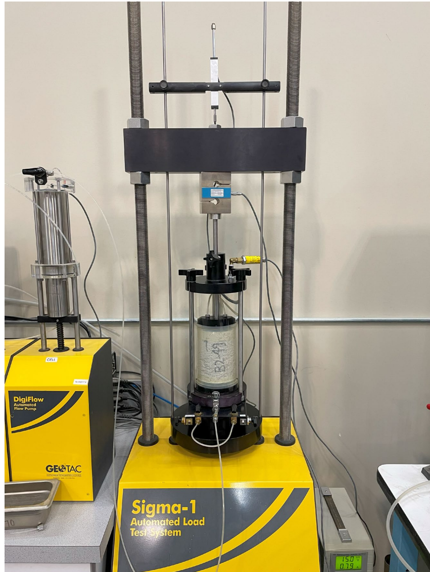
Figure 11-1 Photo of the triaxial testing apparatus with a test specimen in the triaxial cell
