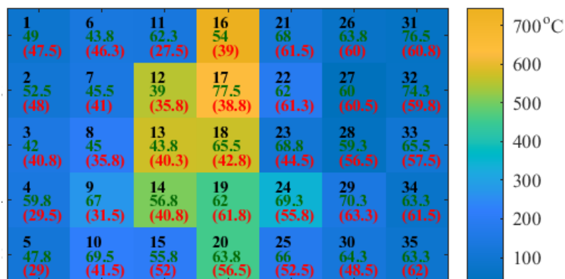
Figure 7.1 Pre-fire and post-fire skid resistance results (green values are pre-fire skid resistance and red values are post-fire skid resistance)
