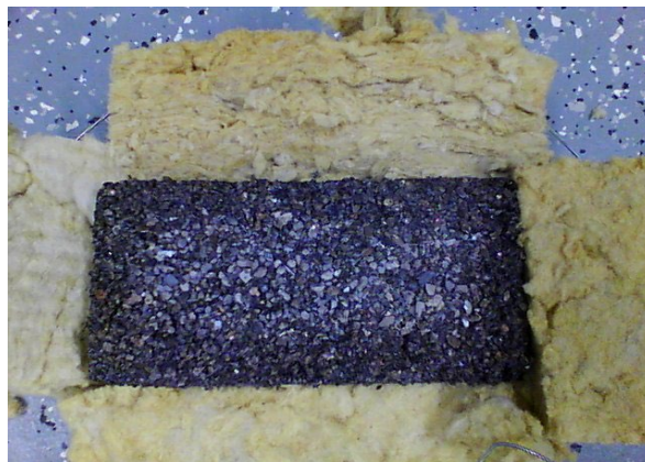
Figure 11.1 Sample with sides insulated to prevent heat input from sides
