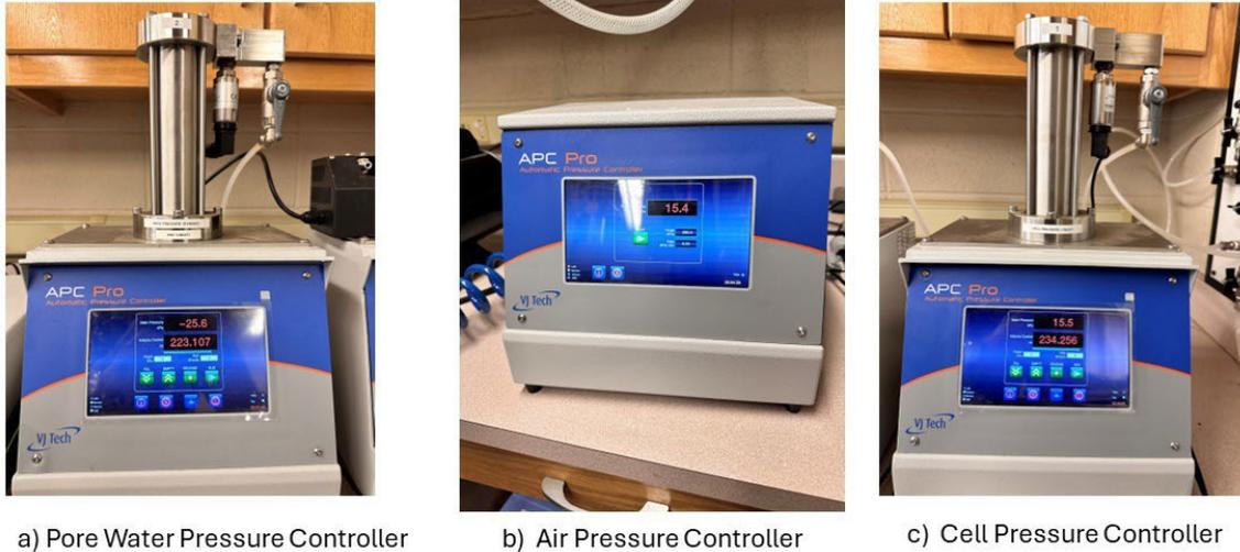
**Figure 3.4** The different pressure units for independent control of overburden pressure and matric suction within a soil sample
