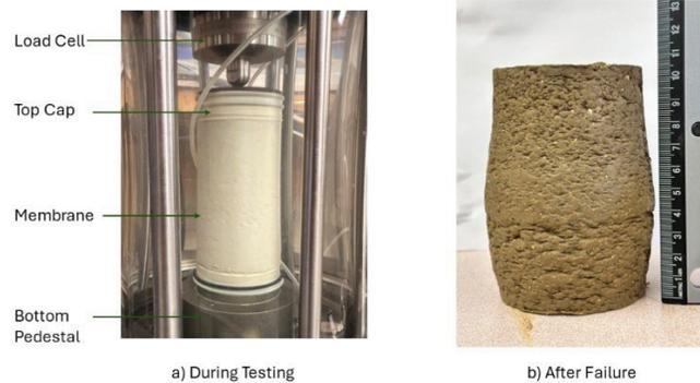
**Figure 3.3** A closer view of the experimental setup and soil sample (a) before and (b) after the completion of a test
