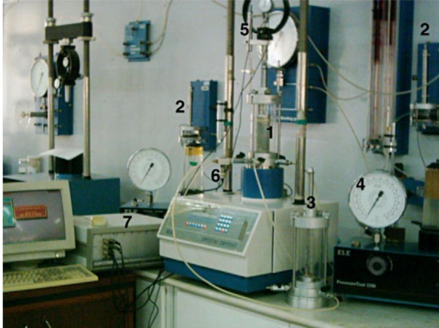
**Figure 2.23** Modified triaxial testing equipment (Kayadelen et al. 2007)
