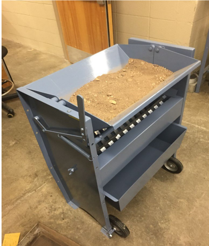
Figure 3.1 Reducing the Sample Size Using an Aggregate Splitter
