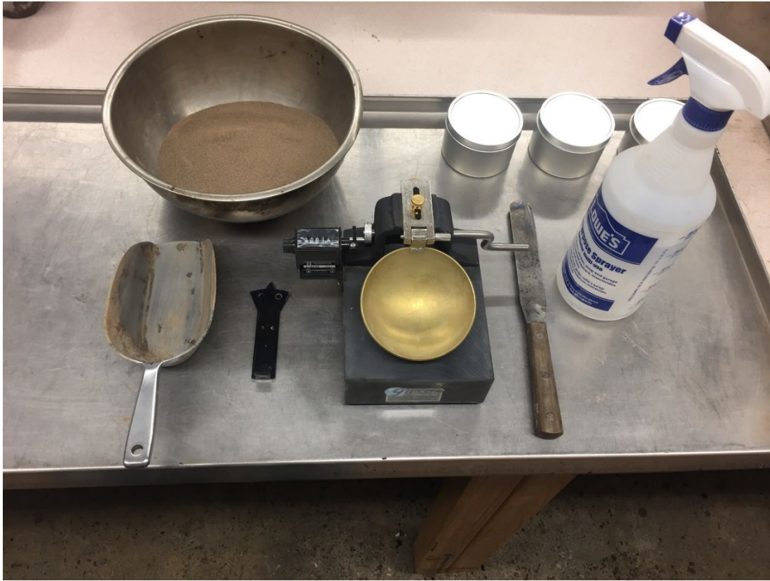
Figure 3.5 A Photographic View of the Test Setup Used for Conducting the Liquid Limit Test
