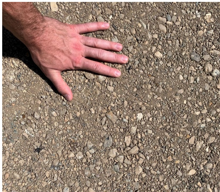
Figure 3.15 A Photographic View of the Surface Texture of a Compacted Aggregate Base (03RQ)
