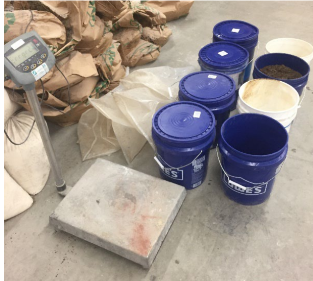
Figure 3.9 Aggregate Base with Optimum Moisture in Sealed Buckets before Compaction
