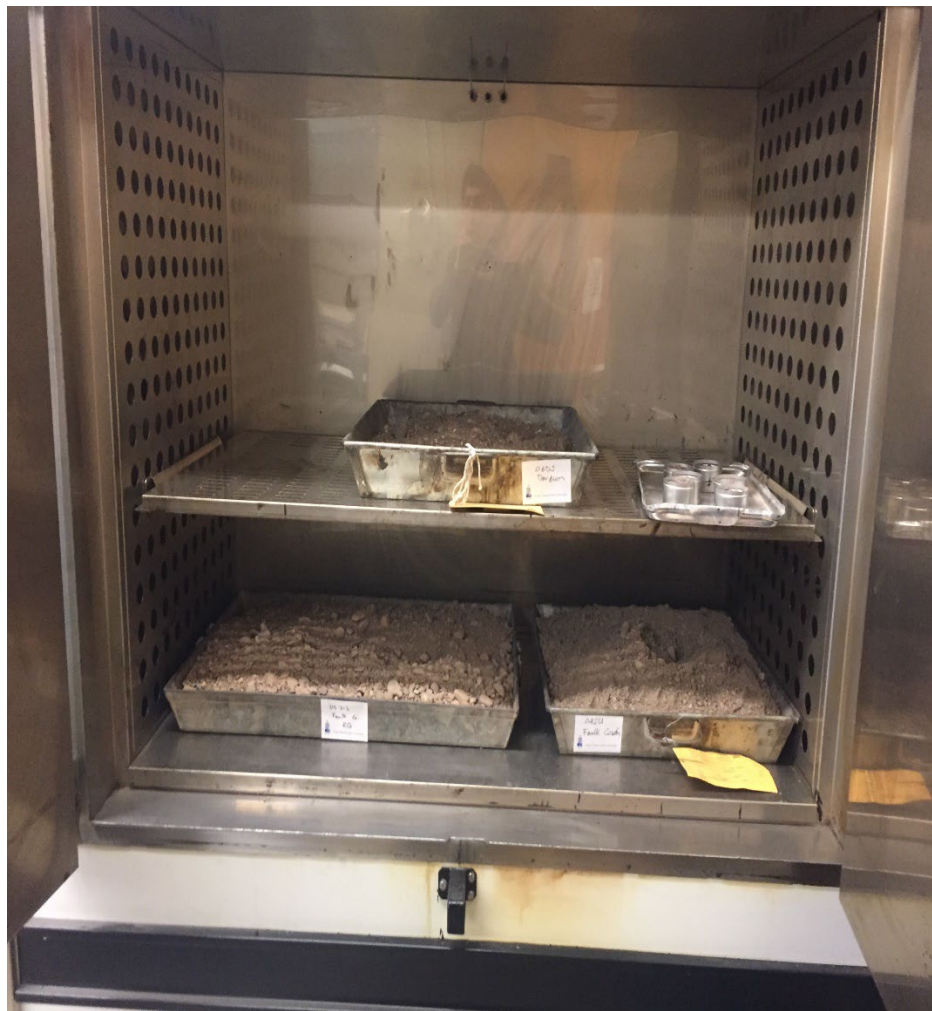
Figure 3.3 Drying Aggregate Samples in an Oven to a Constant Mass
