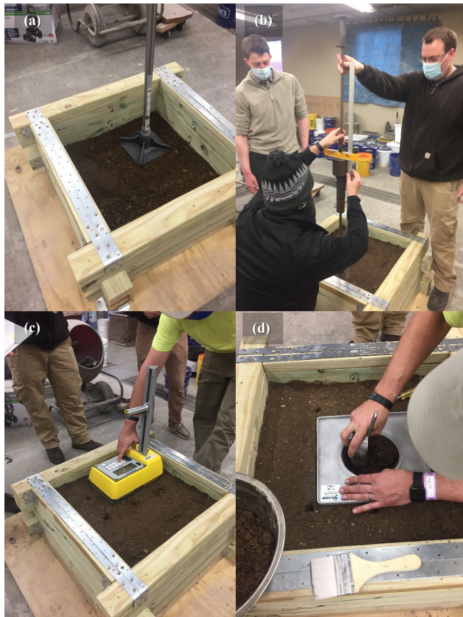
Figure 3.11 Photographic Views of (a) Compacting 042U Base; (b) DCP; (c) NDG; and (d) SCT
