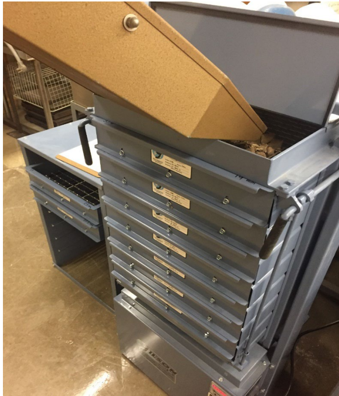
Figure 3.4 An Aggregate Sample being Poured into a Sieve Nest in a Sieve Shaker
