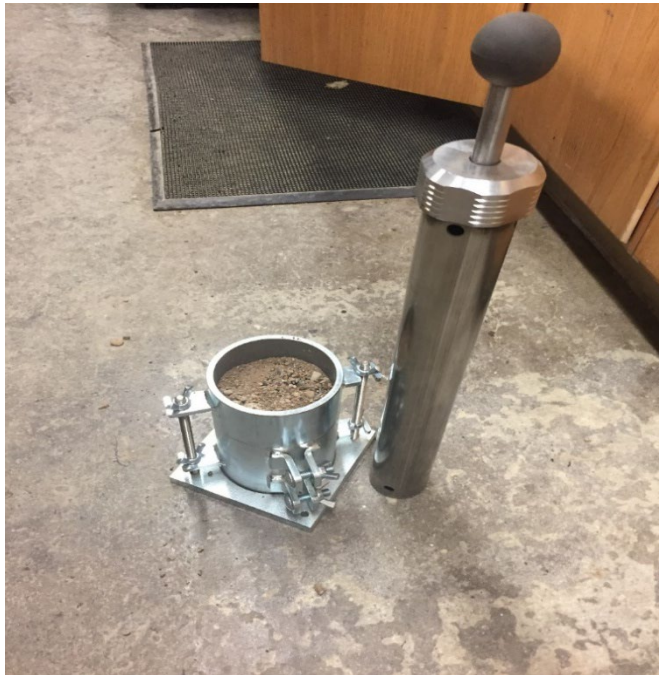
Figure 3.2 Photographic View of an Aggregate Sample in Proctor Mold and Compaction Rammer
