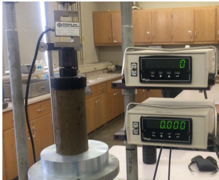
Figure 3.10 Specimen tested for unconfined compressive strength
