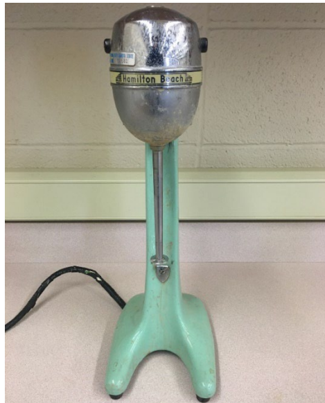
Figure 3.15 Hamilton Beach dispersion device used to thoroughly mix soil slurry
