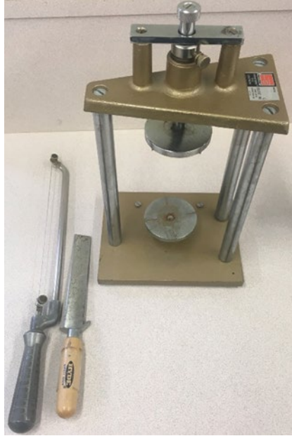
Figure 3.8 Device and tools used to trim soil specimen
