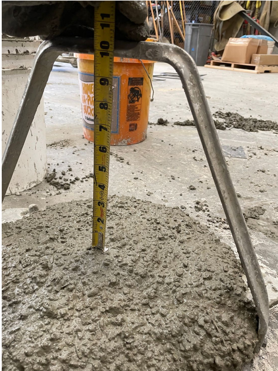
Figure B.1 Photo of Slump Test
