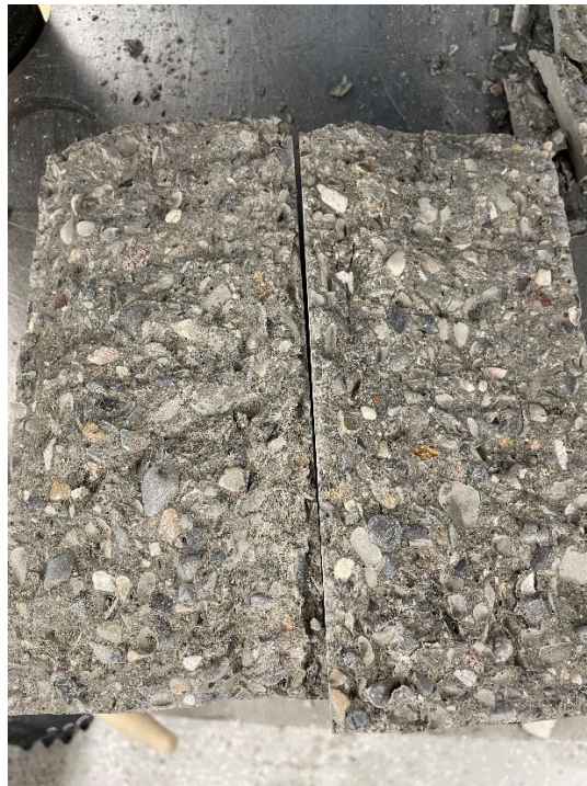
Figure 3.16 Plain Concrete Cylinder Failed During Tensile Test
