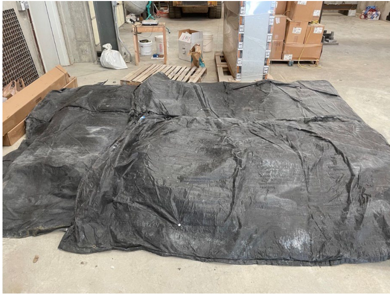
Figure B.7 Insulated Tarp over Concrete Specimens
