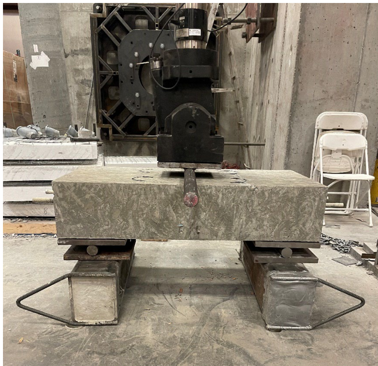
Figure 3.28 Testing Setup for Ultimate Strength Analysis
