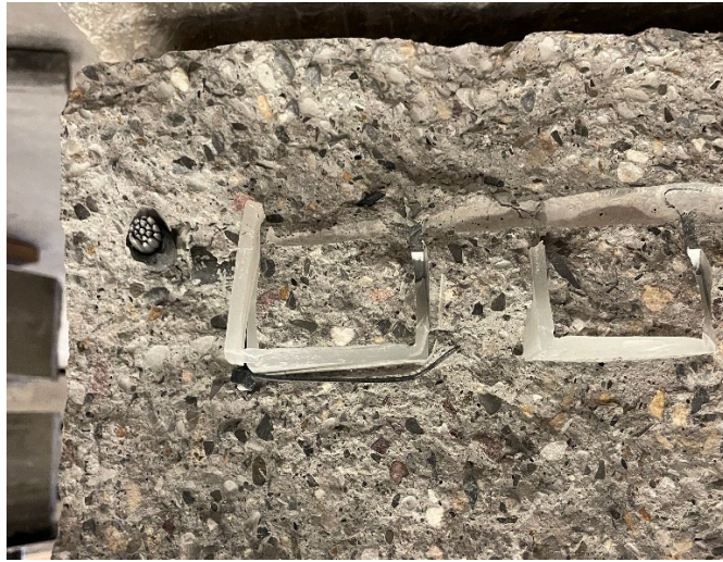
Figure 5.21 Control Slab Exposed Failure Plane
