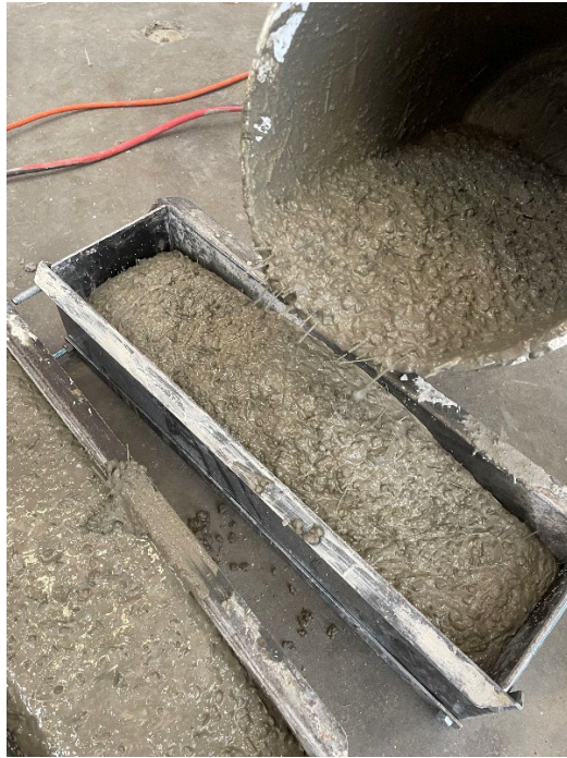
Figure B.4 Filling the Mini-Beam Molds with FRC
