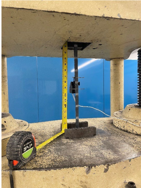
Figure 3.21 FRP Grid Tensile Testing Setup
