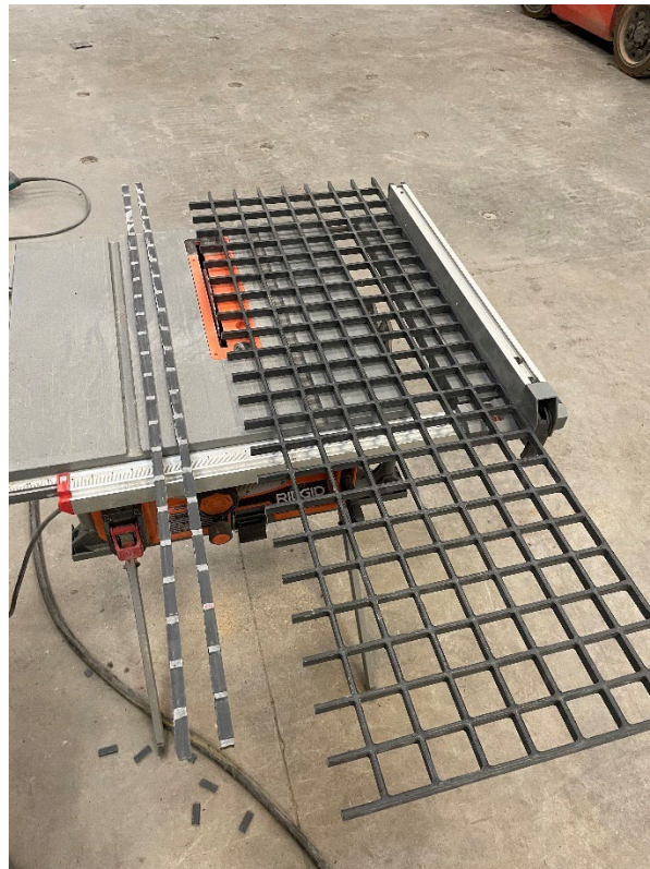
Figure B.8 Cutting Linear Testing Specimens from the FRP Grid
