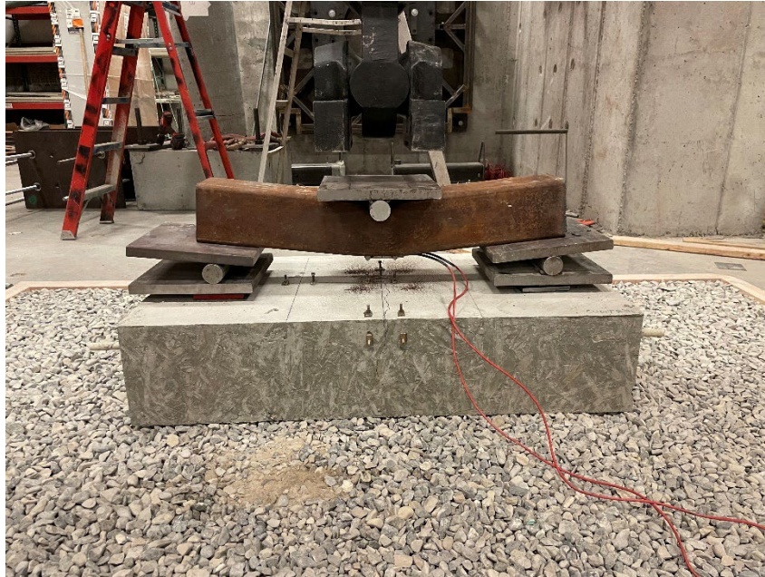
Figure 5.9 Control Slab Spreader Beam Failure
