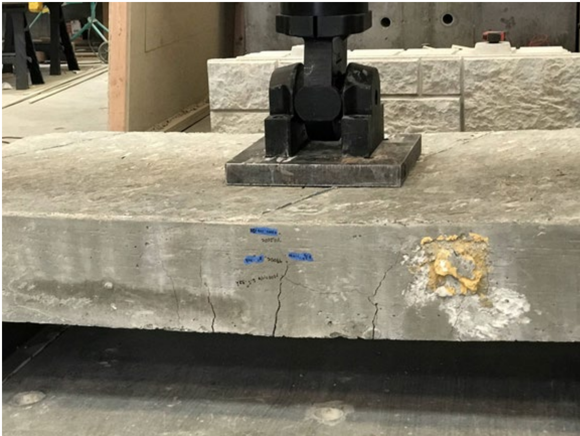
Figure 5.19 Cracking During Static Test
