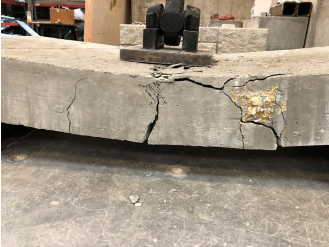
Figure 5.8 Steel Cracking at Midspan
