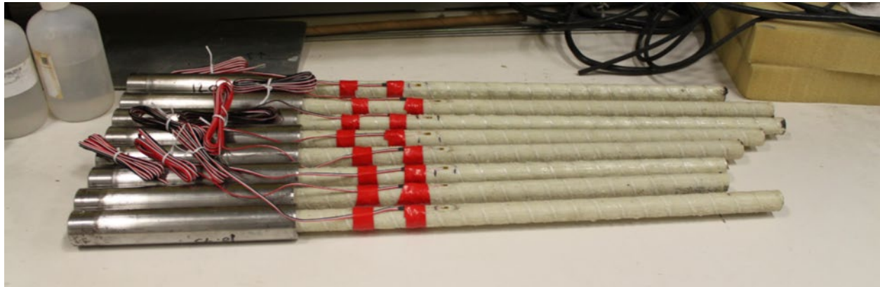
Figure 2.4 Prepared bars with strain gauge installed
