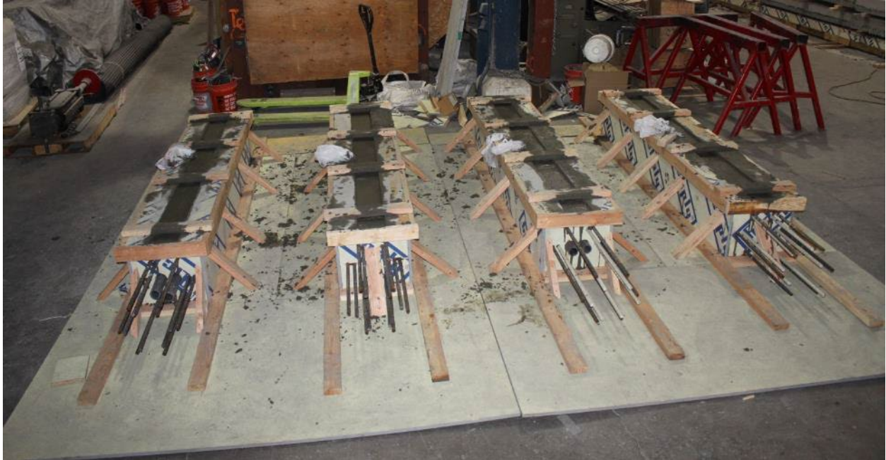
Figure 2.16 Column concrete casting
