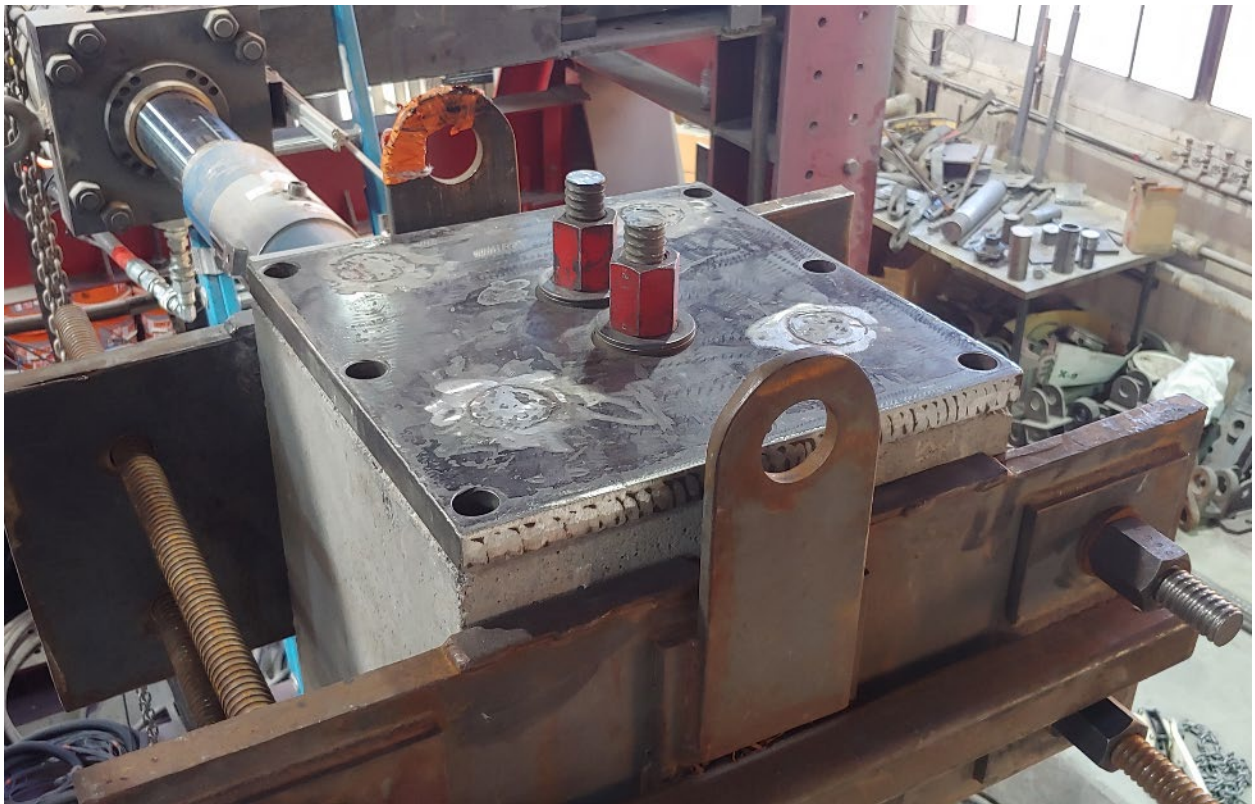
Figure 2.21 PT bars were installed before setting the axial load mechanism
