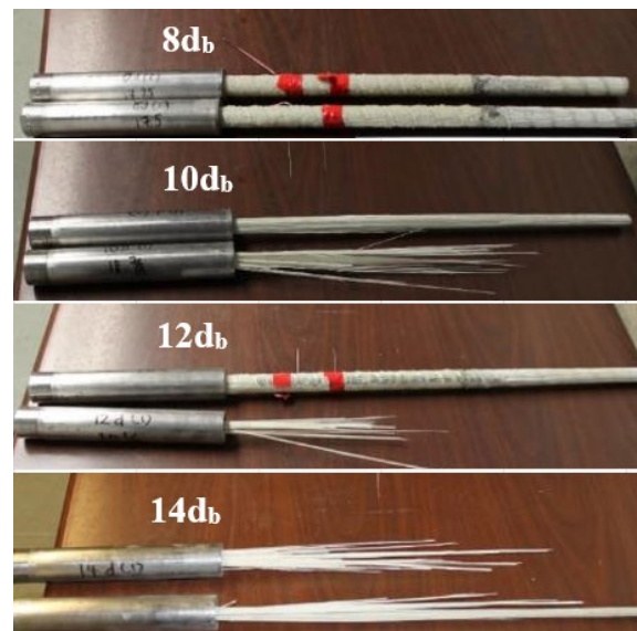
Figure 2.7 Bar failure after tests: 8db as bond failed (bar slipped out), 10db, 12db, & 14db as bar fractured
