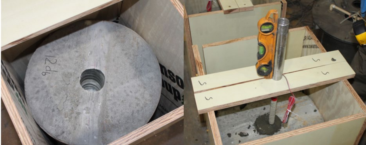
Figure 2.5 Typical specimens before and after bar embedded
