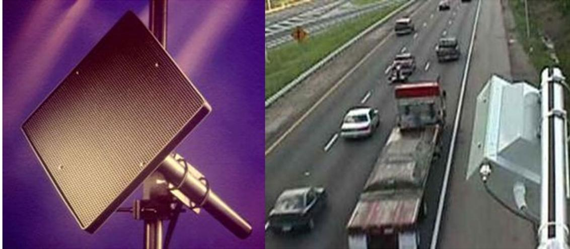
**Figure 2.6** Acoustic Sensors
