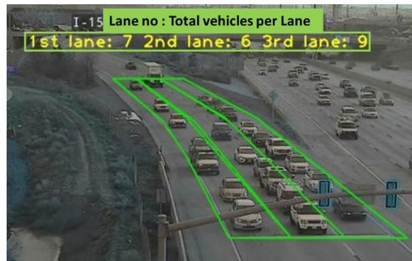
**Figure 3.12** Queue Length Detection Using Image Processing
