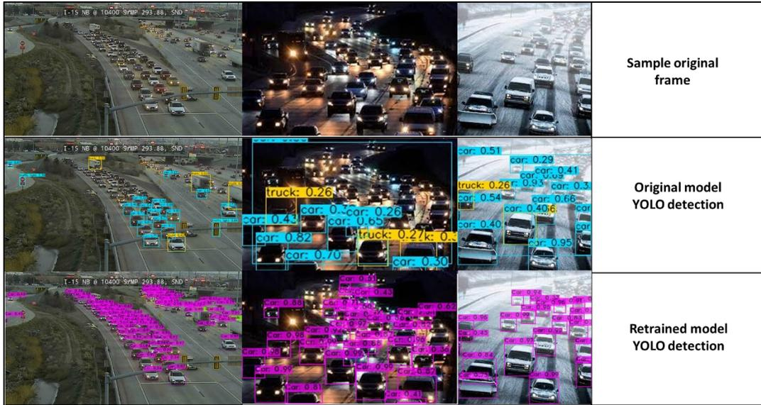
Figure 4.2 Comparison of Base YOLO Model and Retrained YOLO Model
