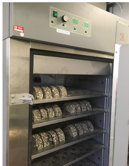
Figure 5.12 Half-Disc Specimens Curing in the Environmental Chamber
