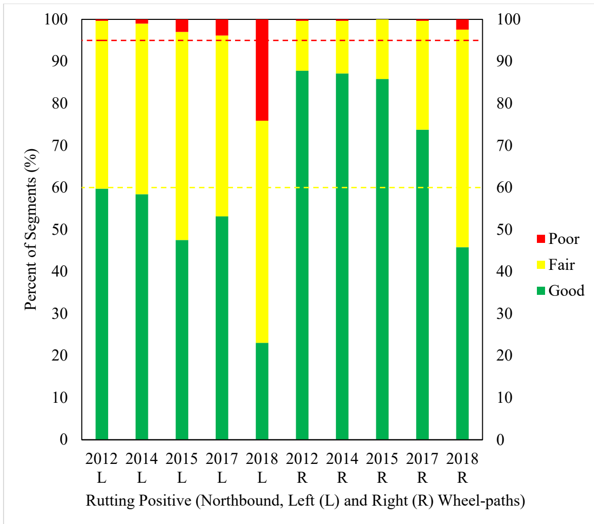
Figure 3.8 Comparison of Right and Left Wheel-Path Rutting for the Positive Direction
