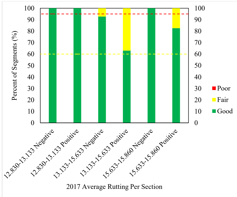
Figure 4.5 Comparison of 2017 Negative and Positive Direction Rutting by Roadway Section
