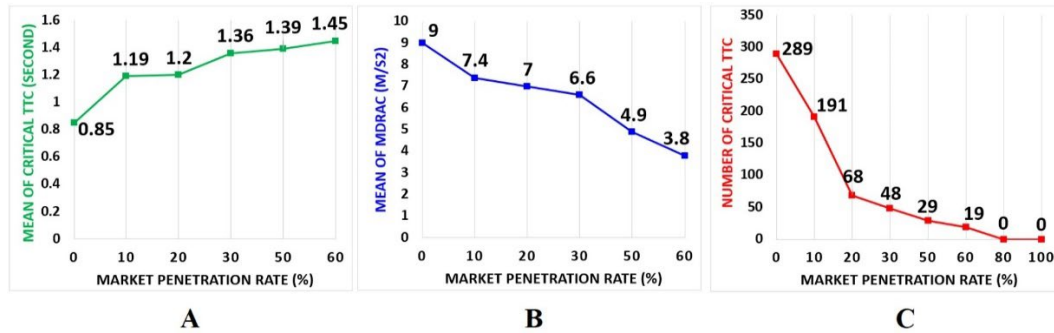
Figure 6.3 Relationship between Conflict-Based Surrogate Measure of Safety (C-SMoS) and Connected Vehicle Market Penetration Rate (CV-MPR)
