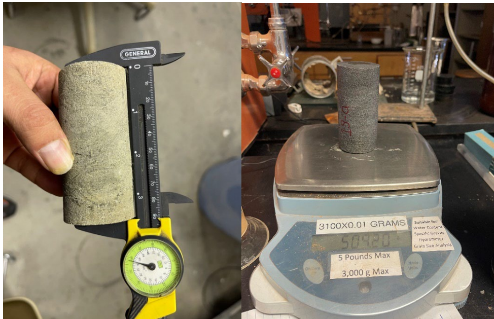
Figure 3.10 Measurement of height, diameter, and weight of each rock specimen
