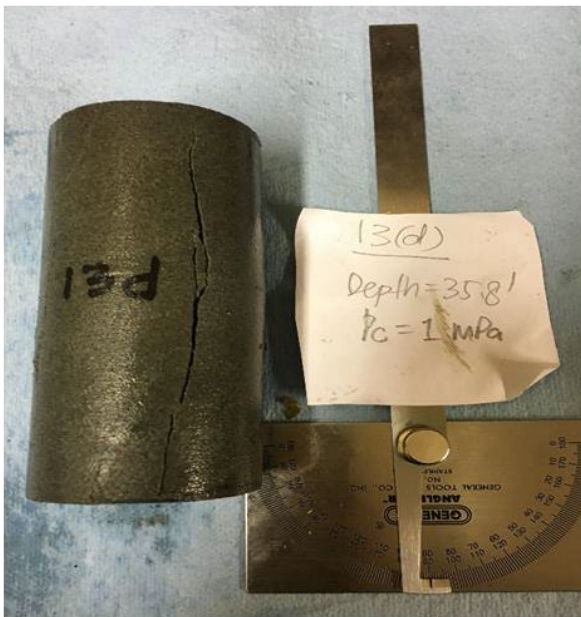
(c) Tensile failure across discontinuities
