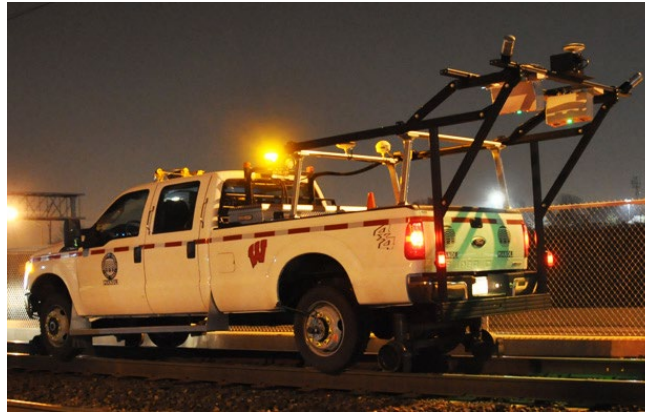
Figure 1.2 Mobile LiDAR for roadway asset data collection (Mandli Communication setup)
