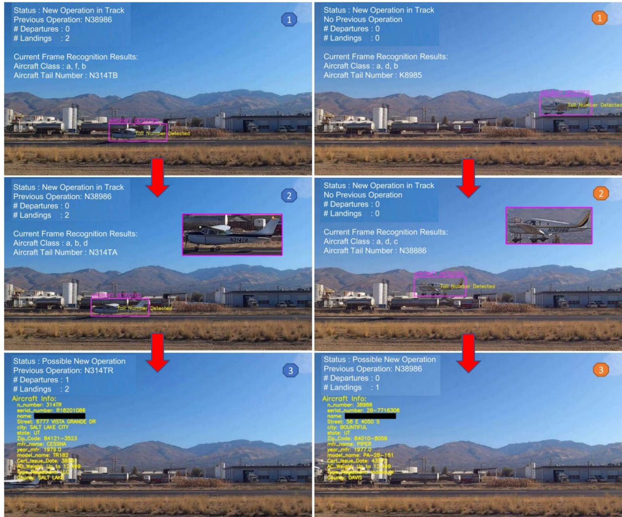
Figure 5.2 AIVATS software performance during (top image) and right after (bottom image) the aircraft operation in layout 1
