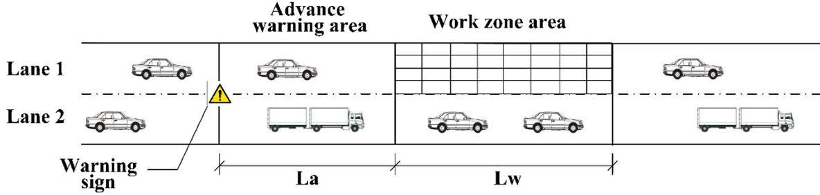
**Figure 2.2** Configuration of a typical work zone
