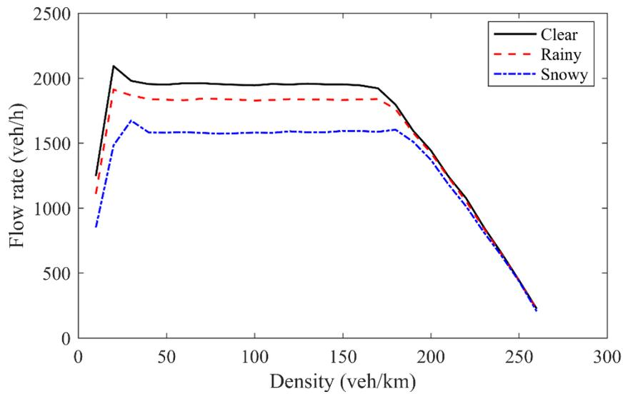
**Figure 3.1** Flow-density diagrams under different weather conditions
