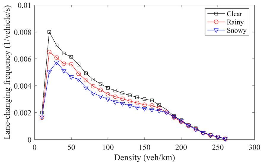
**Figure 3.3** Lane-changing frequency under different weather conditions
