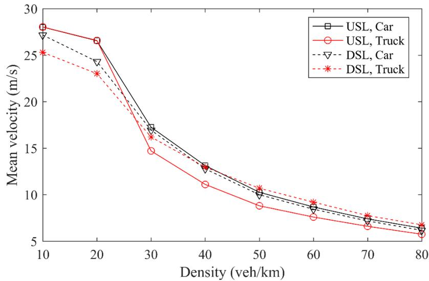
**Figure 3.10** Mean velocity of cars and trucks under USLs and DSLs during rainy weather
