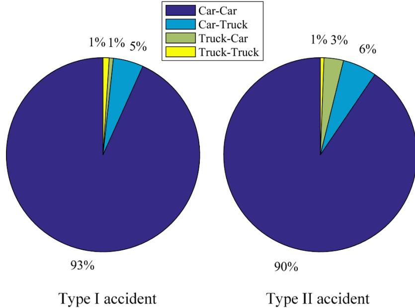
**Figure 3.5** Proportion of MVCs involved different vehicle types under snowy weather
