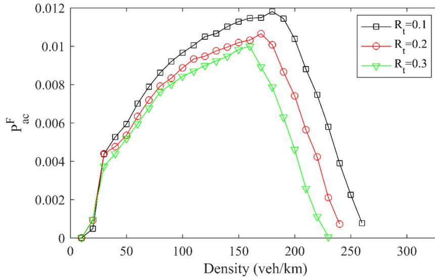
**Figure 3.13** Type I MVC probability for different truck ratios in snowy weather
